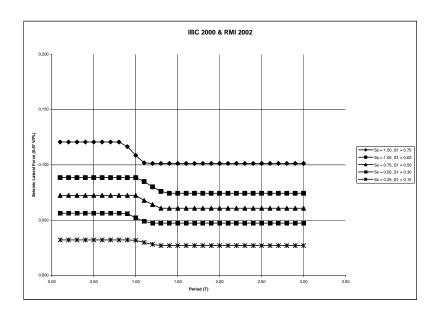
Figure 4-3 Determining seismic coefficients using IBC 2000 Sec. 1622.3.4 (the RMI standard with additional requirements).
