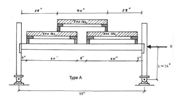
Figure 6-3 Portal tests – loading arrangements (Krawinkler et al. 1979).
