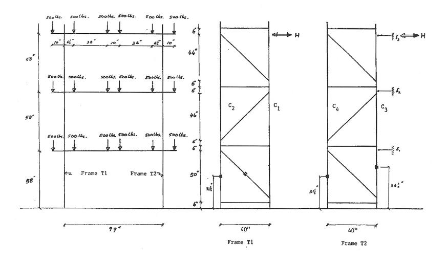
Figure 6-7 Loading summary and instrumentation – Test A-R-2 (Krawinkler et al. 1979)
