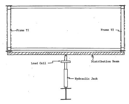
Figure 6-5 Experimental set-up – transverse tests (Krawinkler et al. 1979).
