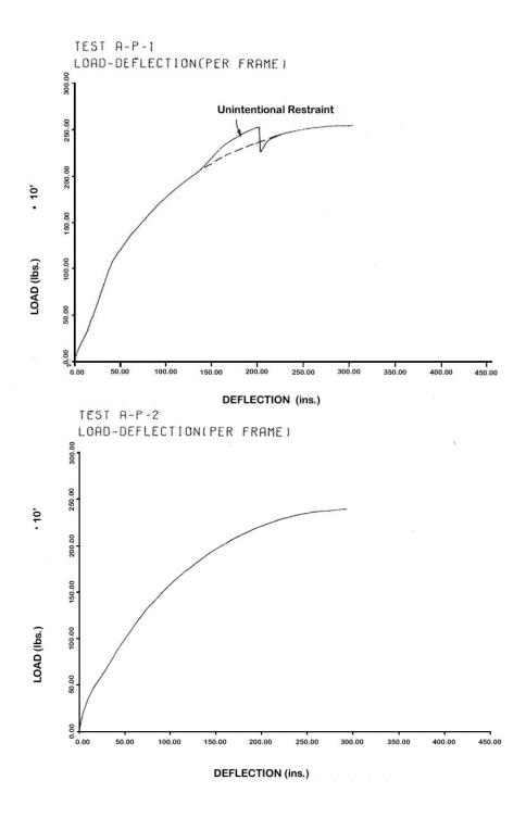
Figure 6-4 Portal tests – H –  $\sigma$  for Rack Type A (Krawinkler et al. 1979).
