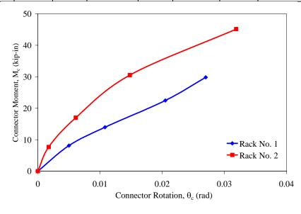
Figure A-5 Envelope of beam-to-upright connector moment-rotation relationship predicted by analytical model.
