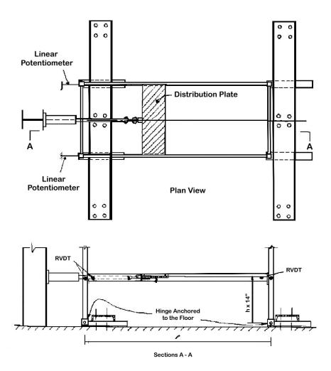
Figure 6-2 Portal test set-up (Krawinkler et al. 1979).
