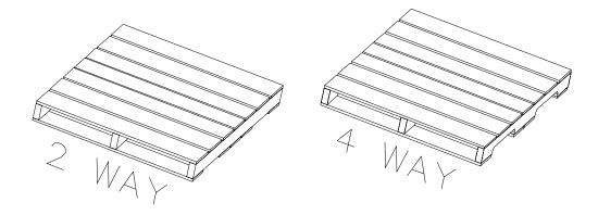
Figure 4.1 Typical pallets used in retail operations.
