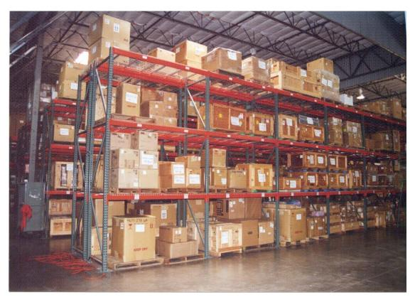
Figure 1-1 Typical steel single selective pallet storage rack.
