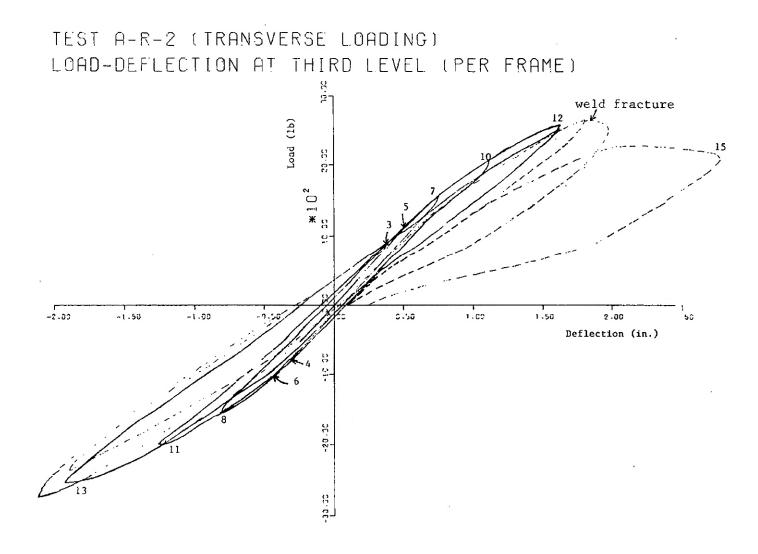
Figure 6-8 Load defelection at third level (per frame) – Test A-R-2, traverse loading (Krawinkler et al, 1979)
