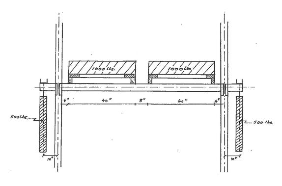
Figure 6-6 Loading arrangements per level per frame – Tests A-R-2 and B-R-2 (Krawinkler et al. 1979).
