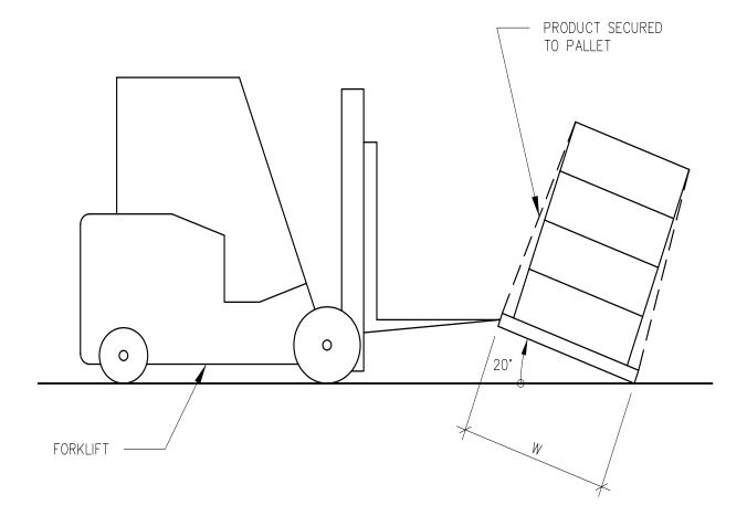
Figure 8-6 The pallet tilt test is used to verify the strength of the means (e.g., stretch wrapping, banding) used to secure merchandise to pallets.
