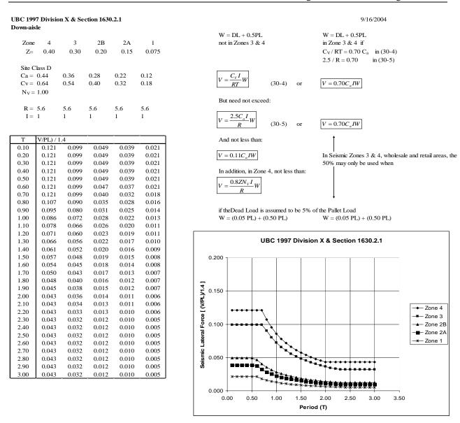
Figure 4-5 Determining seismic coefficients using UBC 1997, Division X.
