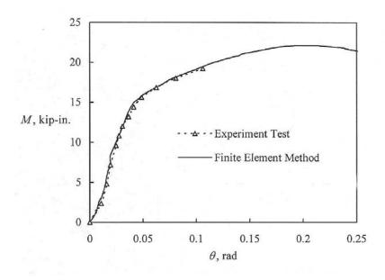
Figure 6-1 Comparison of the cantilever test and the analytical model (from Sarawit et al. 2003).
