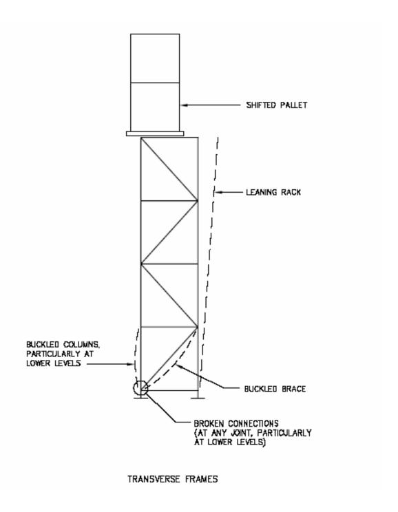
Figure 12-2. Indicated above are the recommended post-earthquake inspection points for cross-aisle (transverse) rack frames. Each frame should be examined.
