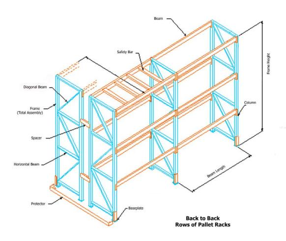
Figure 1-2 Typical storage rack configuration.
