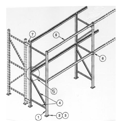
Figure 12-3 Inspection points for an ATC-20 detailed evaluation of a rack. Numbers refer to the inspection points listed above.
