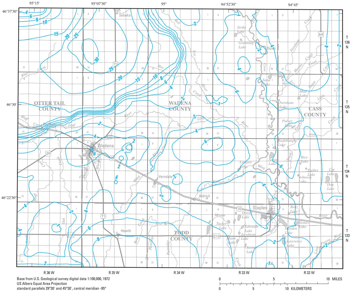
**Figure 17b.** Simulated drawdowns for model layer 3, representing the uppermost confined aquifers due to anticipated increased ground-water withdrawals and drought conditions, steady-state simulation, southern Wadena County and parts of surrounding counties, Minnesota.
