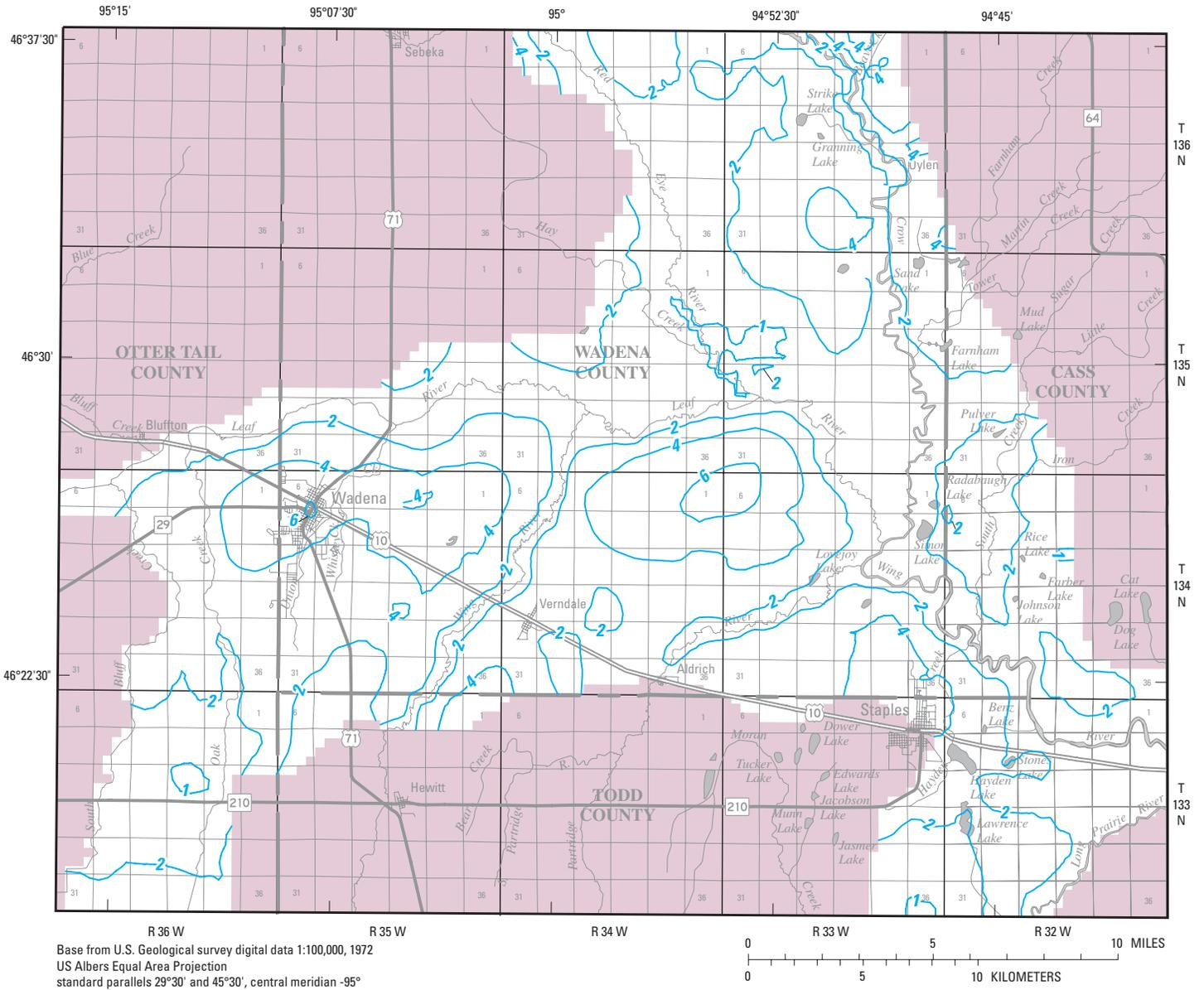
**Figure 17a.** Extent of surficial aquifer and simulated drawdowns for model layer 1, representing the surficial aquifer, due to anticipated increased ground-water withdrawals and drought conditions, steady-state simulation, southern Wadena County and parts of surrounding counties, Minnesota.
