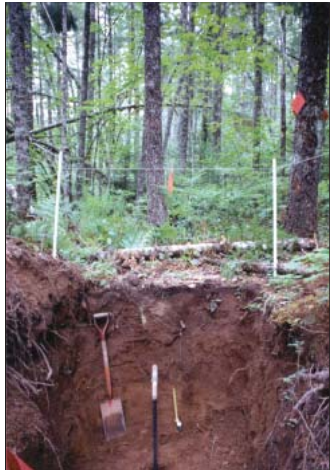
Figure 21—Depth to bedrock was determined by (A) excavation (pit 1 SE to 8.4 ft) or (B) partial excavation and boring (pit 17 NE).
