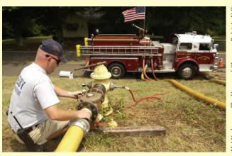
A Shelby firefighter checks a setup whereby a fire truck is used as a pumping station to pump 870 gallons of water per minute from the Shelby municipal water supply through a fire hydrant connected to the Cleveland County water system to a Kings Mountain pumping station 8,000 feet away.
