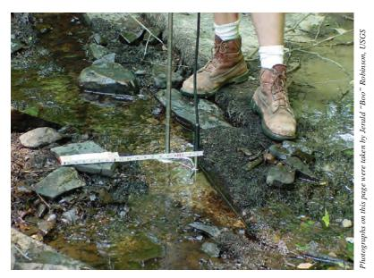
Streamflow measurement being made near USGS streamgaging station at Big Bear Creek near Richfield (site 90, table 4), June 19, 2002.
