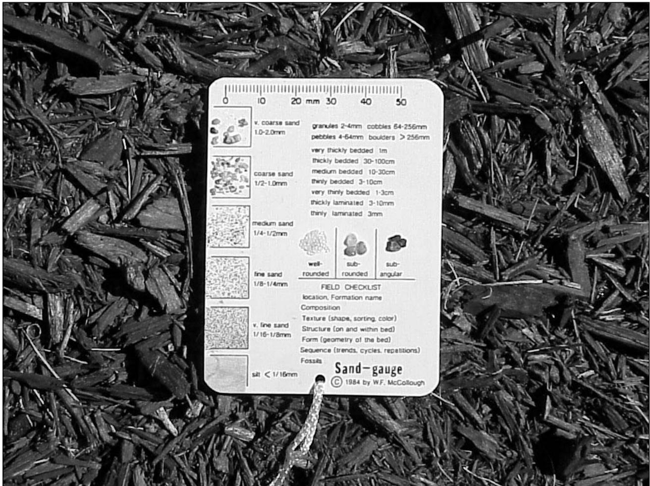
Figure 10. Sand-gauge card used for visual estimation of sediment particle size. (Photograph by P.J. Cinotto, USGS)
