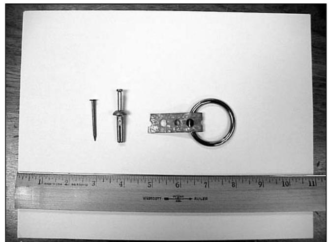
Figure 42. Mounting hardware for sandbag and optical-brightener samplers. (Photograph by P.J. Cinotto, USGS)
