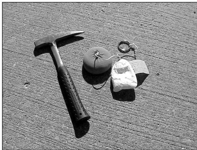
Figure 39. Sandbag and optical-brightener samplers (pick for scale). (Photograph by P.J. Cinotto, USGS)
