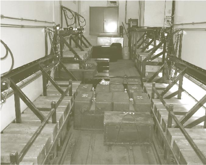
**Figure 16.** *The Netherlands: dynamic calibration vehicle.*
