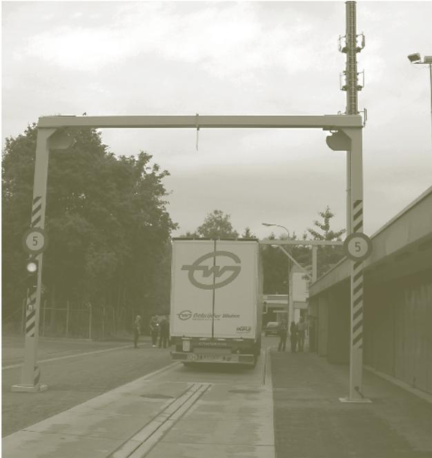
**Figure 10.** *Switzerland: vehicle profiler system.*
