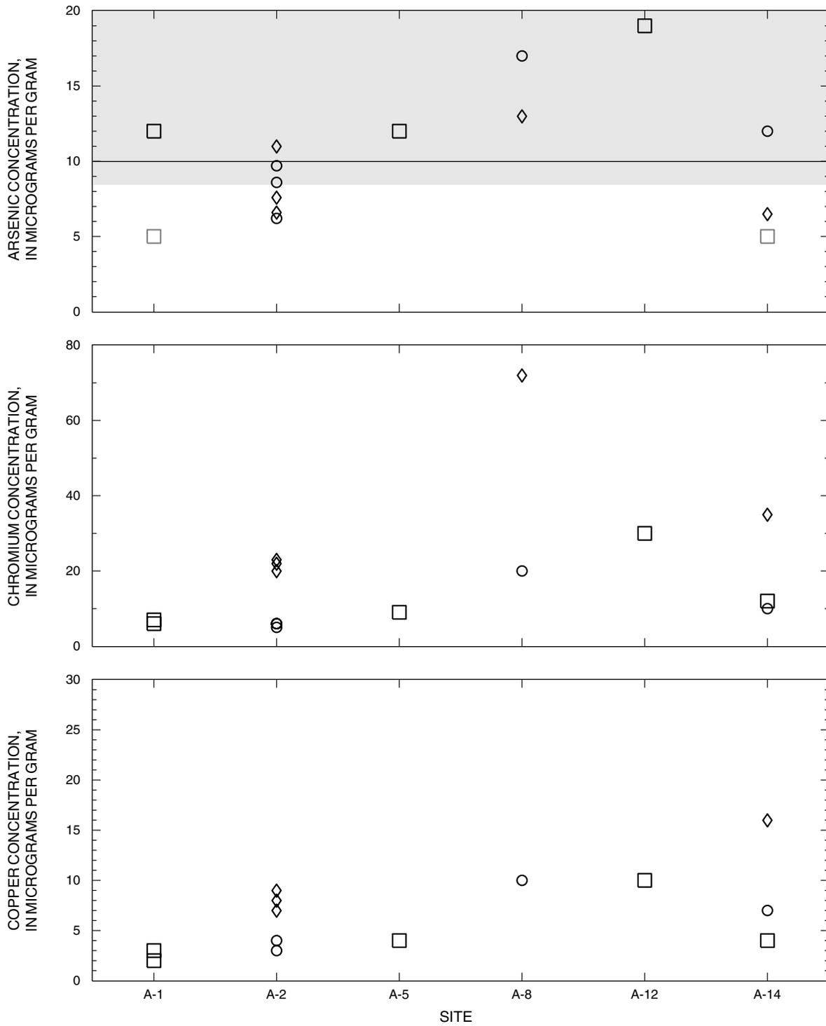
**Figure 9.** Concentrations of selected trace elements in bottom-sediment samples collected from sites in or near the Angostura Reclamation Unit in 1988 and 1994.
