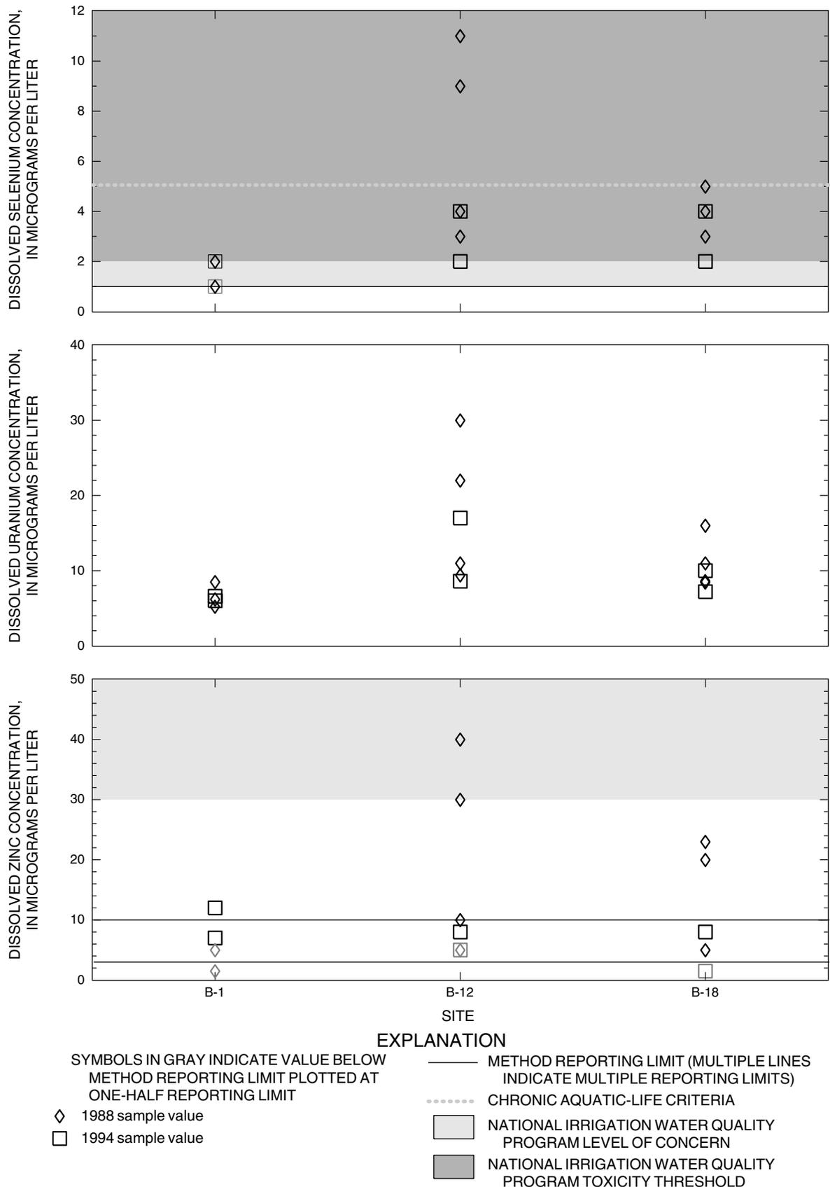
**Figure 11.** Concentrations of selected trace elements in water samples collected from sites in or near the Belle Fourche Reclamation Project in 1988 and 1994. --Continued
