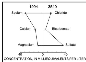
**Figure 6.** Stiff diagrams showing average dissolved-solids concentrations and proportions of major ions in water samples collected from sites in or near the Angostura Reclamation Unit in 1988 and 1994.
