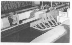
Model of Lock and Dam No. 1 on the Mississippi River built by Waterways Experiment Station
