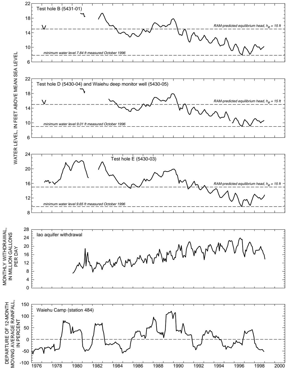
**Figure 12.** Water levels at Waiehu deep monitor well and test holes B and E, departure of backward-looking 12-month moving average rainfall from the long-term average rainfall for Waiehu Camp rain gage, and monthly mean total withdrawal from the lao aquifer prior to 1999, Maui, Hawaii. (Unpublished rainfall data from Commission on Water Resource Management.)
