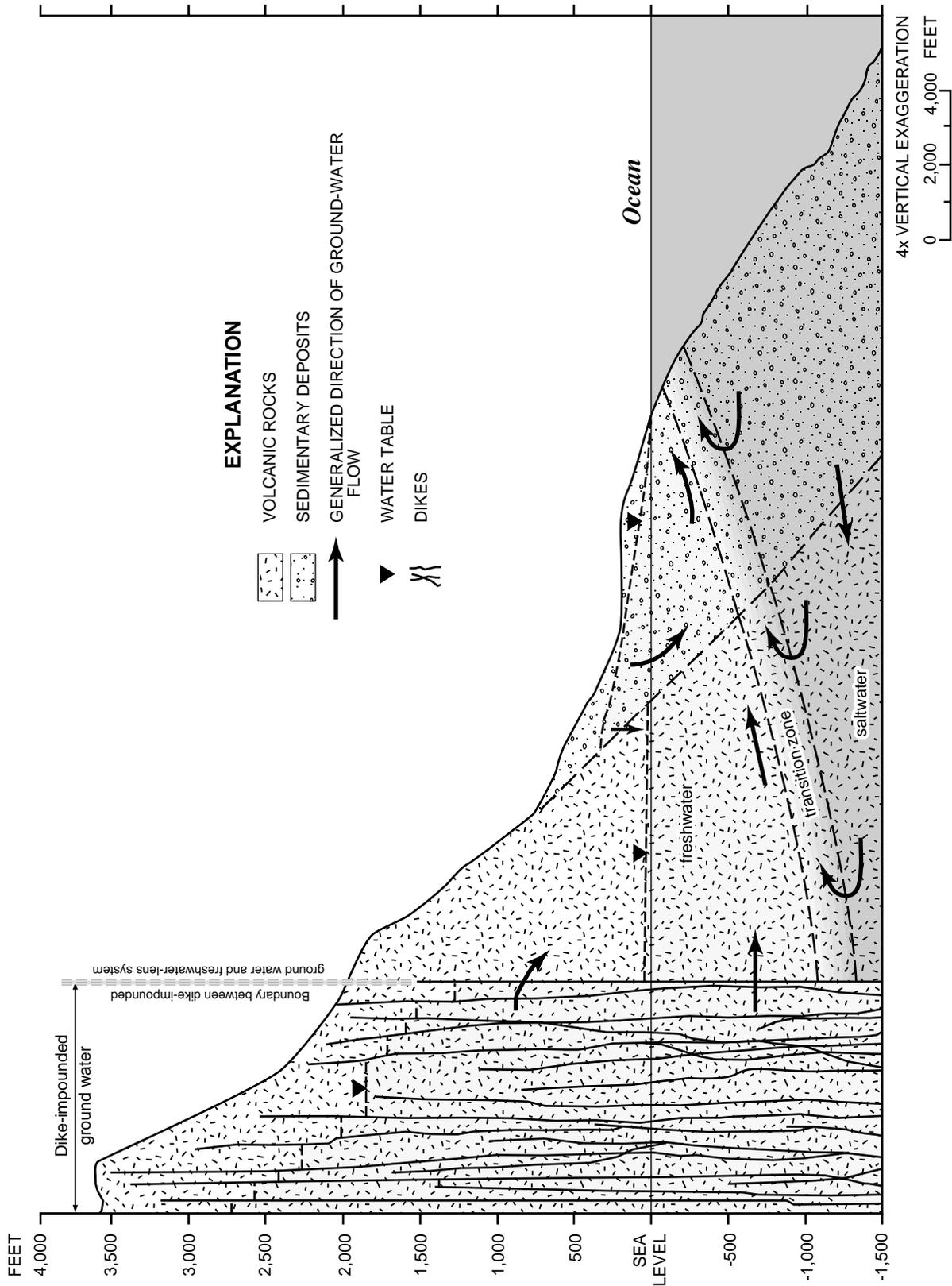
**Figure 1.** Schematic cross section of the regional ground-water flow system of the Iao aquifer, Maui, Hawaii.
