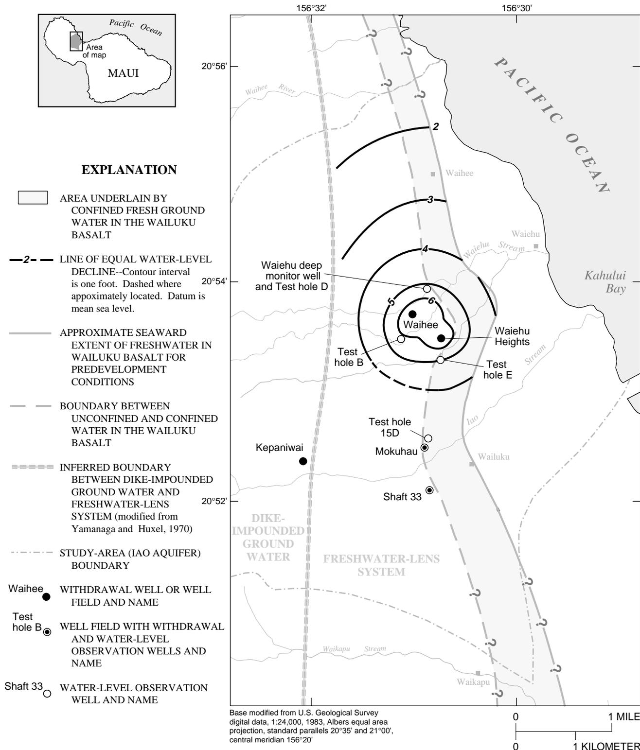
**Figure 13.** Map showing water-level declines in the flank flows of Wailuku Basalt between April 1977 and April 1997 for the northern part of the Iao aquifer, Maui, Hawaii.
