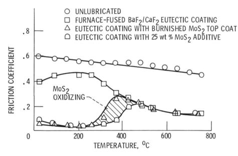
Figure 1. - Effect of  $MoS_2$  as a burnished top coat and as an additive to  $BaF_2/CaF_2$  eutectic furnace-fused coatings. Dry air atmosphere, 2.3 m/s, 500-gram load cast Inconel rider, Inconel 750 disks with 0.004 cm coatings.
