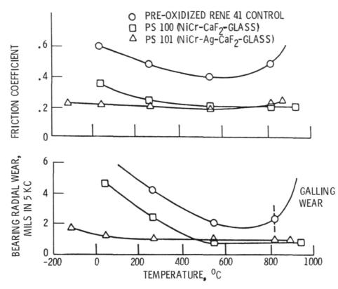
Figure 5. - Effect of silver addition on the friction and wear of plasma-sprayed, nichrome-matrix coatings (from Ref. 12). Lubricating plain spherical bearings at a radial load of 34 MPa. Bearing material, precipitation hardened nickel-chromium alloy.
