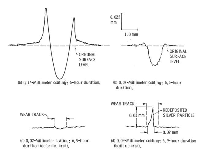
Figure 10. - Wear track cross sections showing effect of coating thickness on wear and deformation of plasma-sprayed silver coatings.
