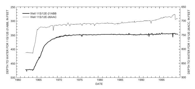
**Figure 40**. Water levels in two wells near Round Butte Dam, showing the rise in ground-water elevations caused by the filling of Lake Billy Chinook.
