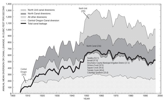
**Figure 10.** Annual canal diversions and estimated annual mean canal leakage in the upper Deschutes Basin, Oregon, 1905–97. (Mean annual discharge, in cubic feet per second, is shown in parentheses for the period of record for each diversion.)
