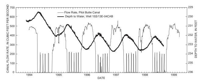
**Figure 36.** Relation between static water-level variations in a well near Redmond, Oregon, and flow rate in a nearby irrigation canal.
