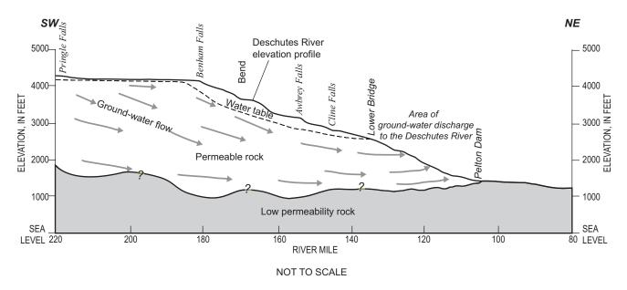
**Figure 18.** Diagrammatic section showing the effect of geology on ground-water discharge along the Deschutes River upstream of Pelton Dam.
