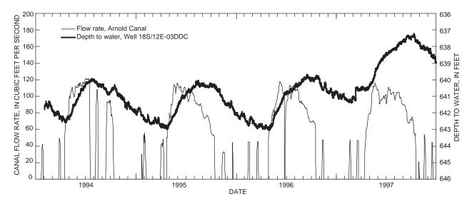
**Figure 35.** Relation between static water-level variations in a deep well near Bend, Oregon, and flow rate in a nearby irrigation canal.
