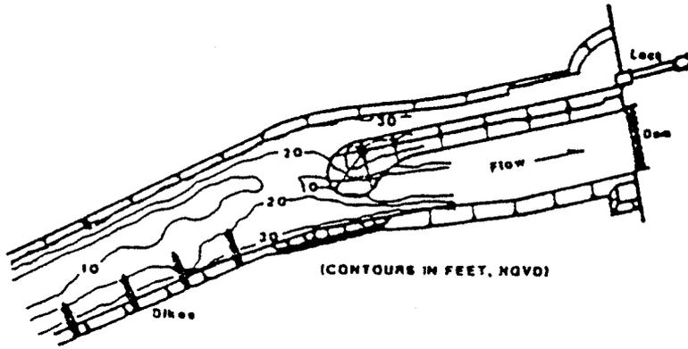
Figure B.3, Bed elevations 20 days after dike construction
