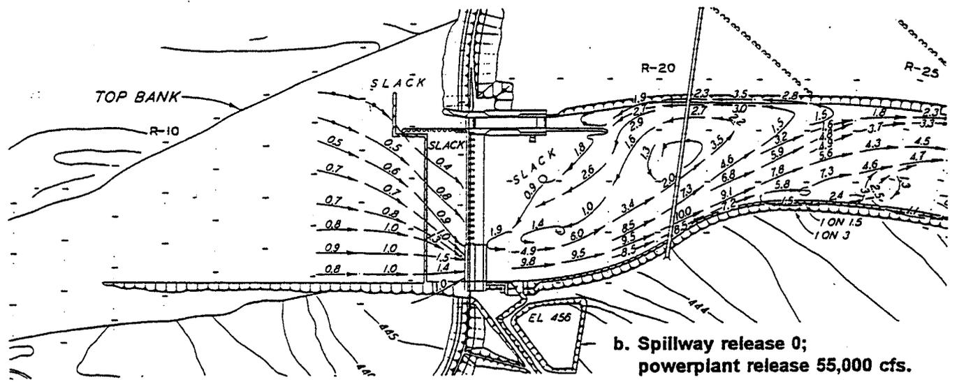
**Figure 9.5. Velocities and currents, original design,
