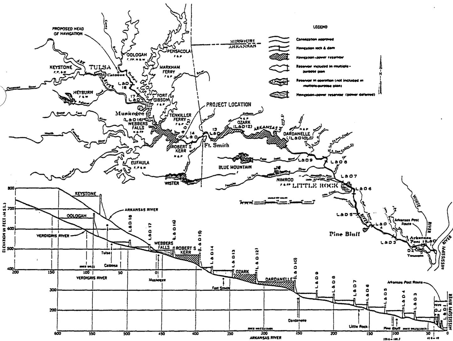
Figure 10.4. Arkansas River Navigation Project (Corps of Engineers).
