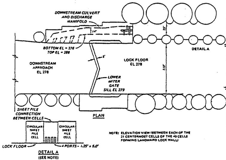
b. Details of lock and discharge culvert.
