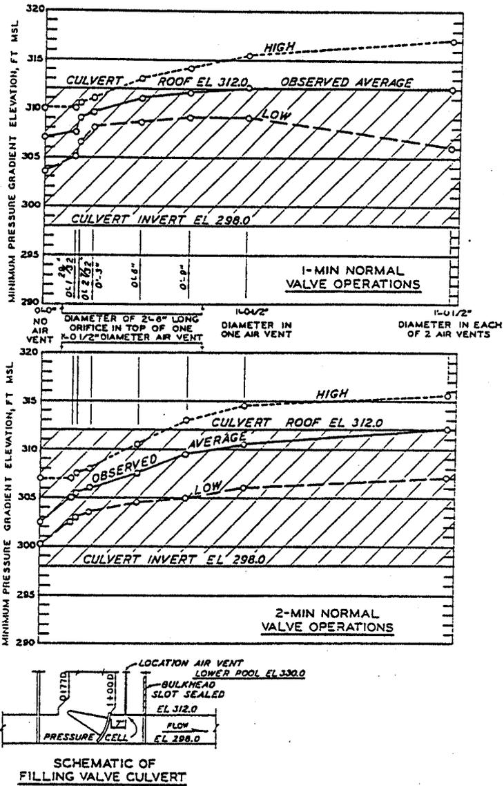
Figure 9.18. Effect of air venting on culvert roof pressures downstream of culvert filling valves, Bay Springs Lock (Ables, 1978).
