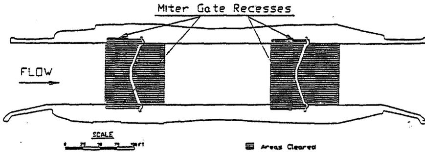
Figure 10.10. Areas cleared of sediment with submersible pump, typical lock, Red River Navigation Project (Neilans, et al., 1993).
