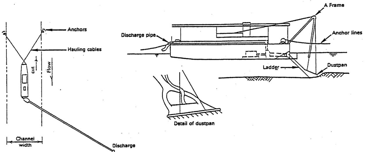
Figure 10.15. Dustpan dredge (U.S. Army, Corps of Engineers).
