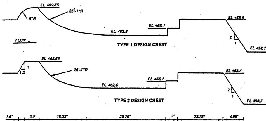
b. Spillway and stilling basin for submersible tainter gate. Alternative spillway crest shapes tested.
