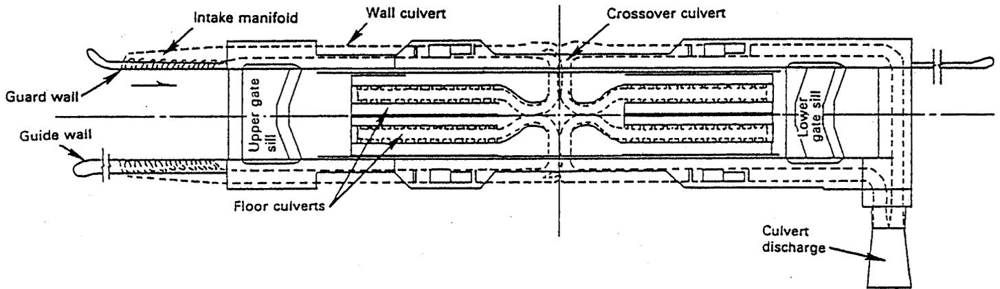
**Figure 8.38. Bottom longitudinal "over-and-under" filling and emptying system, Bankhead Lock, 69-ft lift, Black Warrior River, Alabama (Murphy, 1980).**
