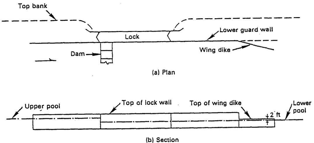
**Figure 9.25. Wing dike to minimize shoaling in lower lock approach, Dardanelle Lock, Arkansas River. (Franco, 1976).**
