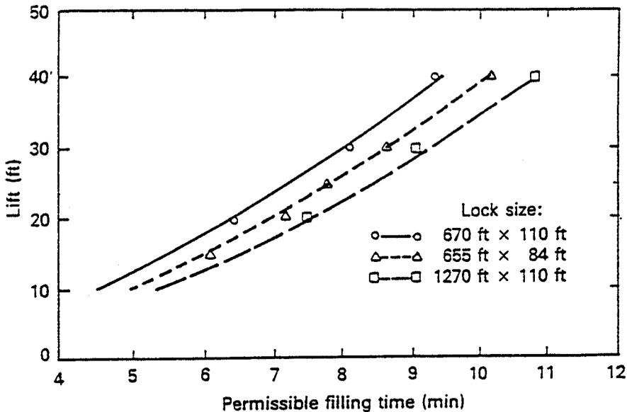
Figure 8.28. Permissible filling times (model) (Murphy, 1975).
