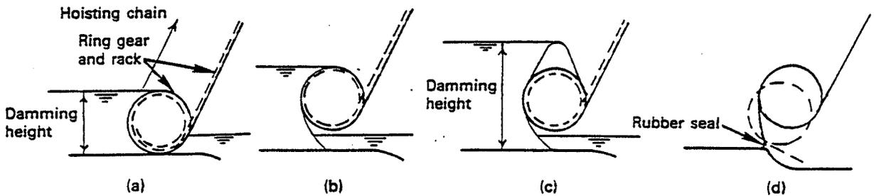
Figure 7.8 Roller gates. (U.S. Army, Corps of Engineers, 1952)
