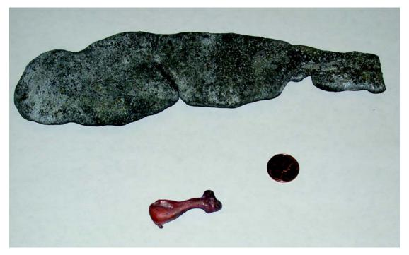
**Figure 6.** Melted aluminum (top) and copper (bottom) recovered from IC 1013 locomotive on northbound train.
