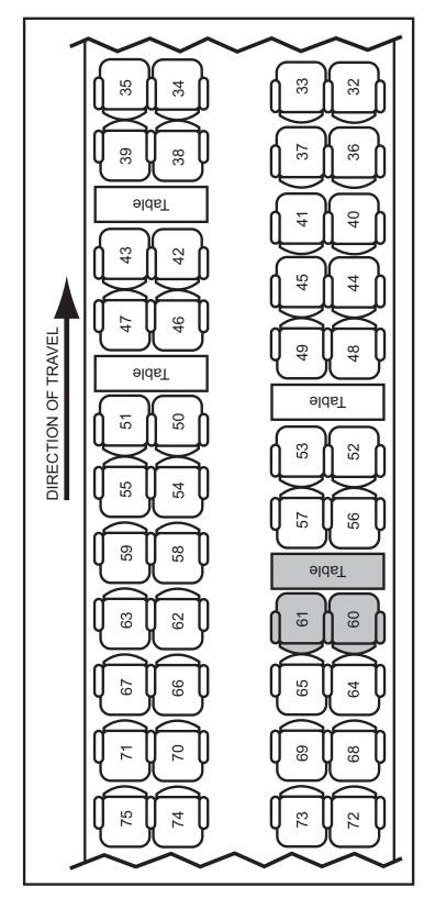
**Figure 7.** Seating layout of the upper-deck level of the Metrolink cab car. (Fatally injured passengers were seated in seats 60 and 61 at workstation table.)
