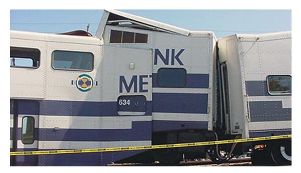
Figure 5. Damaged exterior of Metrolink cab car.
