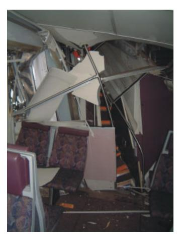
Figure 4. Damaged stairway in Metrolink cab car.
