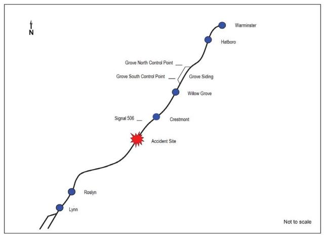
Figure 1. Map of a portion of the Warminster Line and the accident location.
