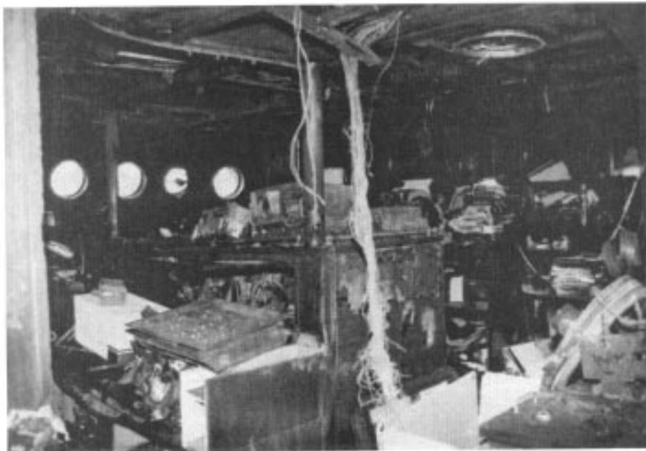
Figure 8 — Fire-damaged wheelhouse, revealing overhead construction
