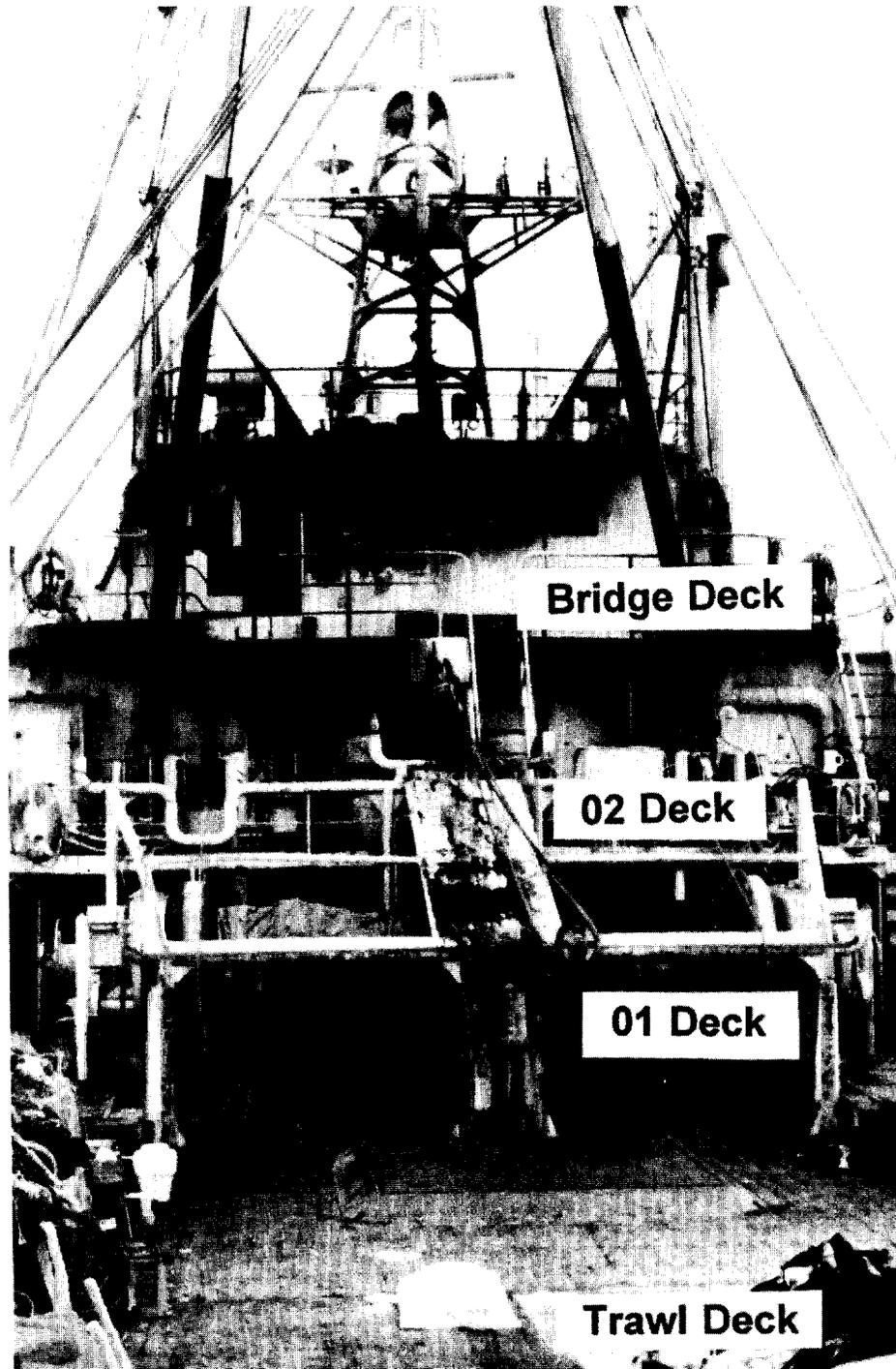
Figure 6 — View of the deckhouse from the trawl deck, looking forward
