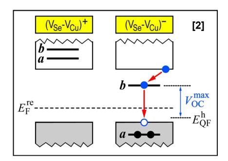
$In_{Cu}$ ,  $Ga_{Cu}$ :  $V_{OC}$  is limited by the transition that causes atomic reconfiguration
