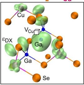
In II-VI, DX centers require **extrinsic** impurities In CIGS, native defects (In<sub>Cu</sub>, Ga<sub>Cu</sub>) exhibit DX behavior
