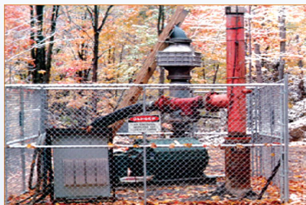
Figure 2: A gob well, used to extract CMM from post-mining collapsed coal seams.
