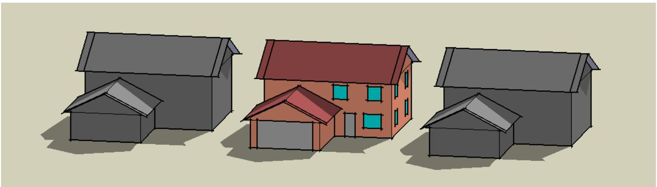
Fig. 3. House geometry with neighboring houses used for shading analysis.
