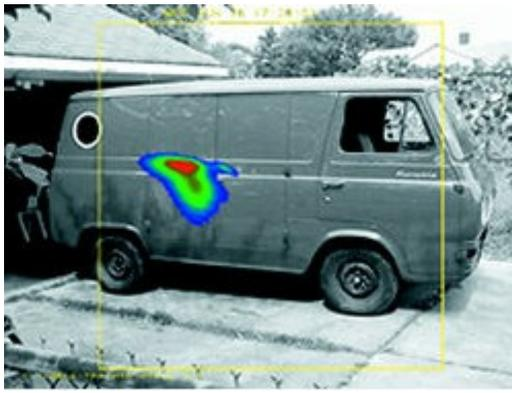
Figure 20. GammaCam<sup>TM</sup> image of a gamma-ray source inside a truck [EDO, 2004].
