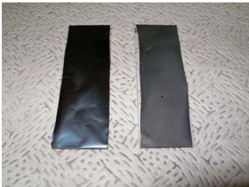
Figure 12. CdTe/CdS/ITO/Al structures with CdTe deposited by PVD (left) and VT (right).
