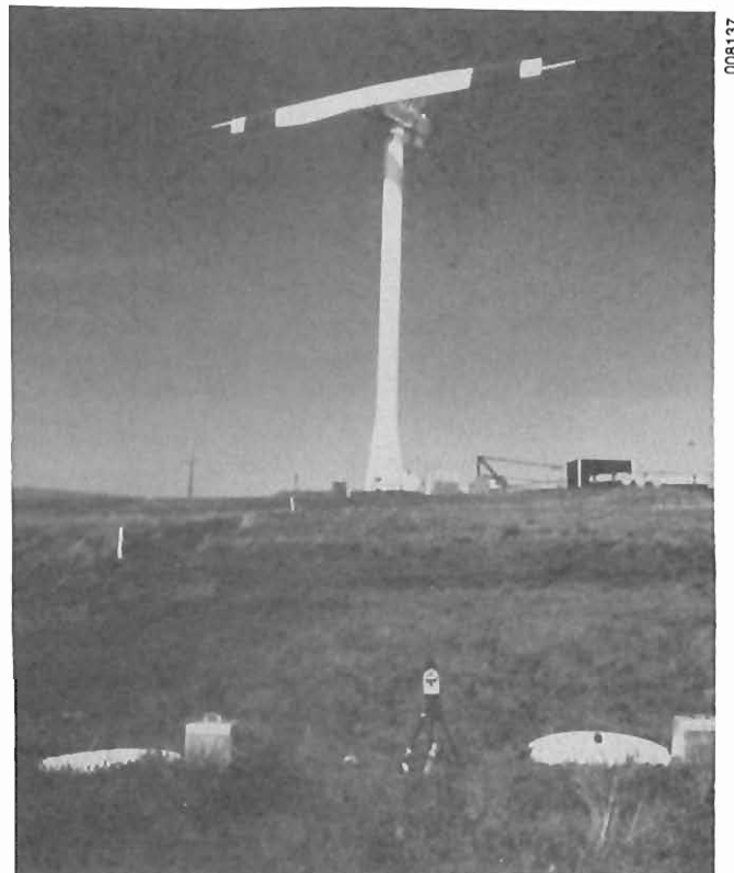
Figure 2-1. Microphone Measurement Station
