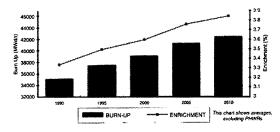
source: Uranium Institute 1992 The graph from Sweden's Oskarsamn-3 reactor shows that with increasing fuel burn-up from 35,000 to 55,000 MWd/t a constant amount of uranium is required per unit of electrical output, and energy used (indicated by SWU) for increased levels of enrichment increases slightly. However, the amount of fabricated fuel used in the reactor drops significantly due to its higher enrichment and burn-up.
