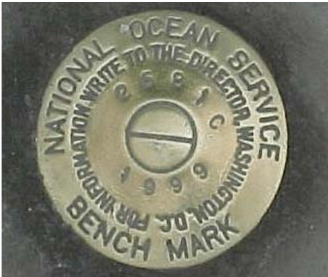
Figure 4.22: Digital Photo of Stamping of Bench Mark
