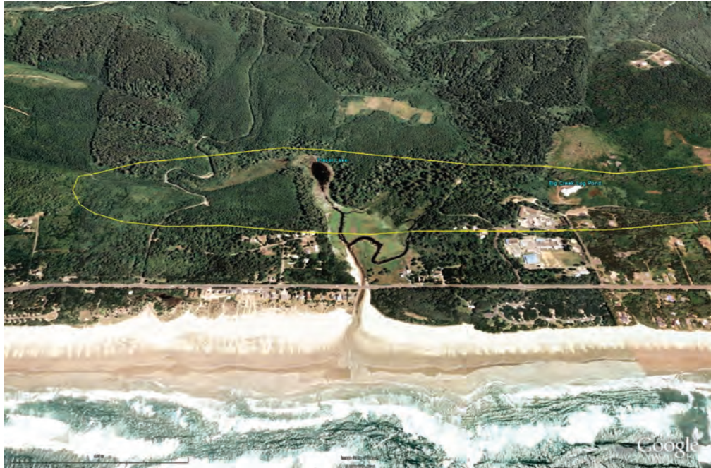
Figure 18. Aerial photo of Placer Lake from Google Earth imagery. Yellow line indicates where SRTM data replaced NED data in building the Central Oregon Coast DEM.
