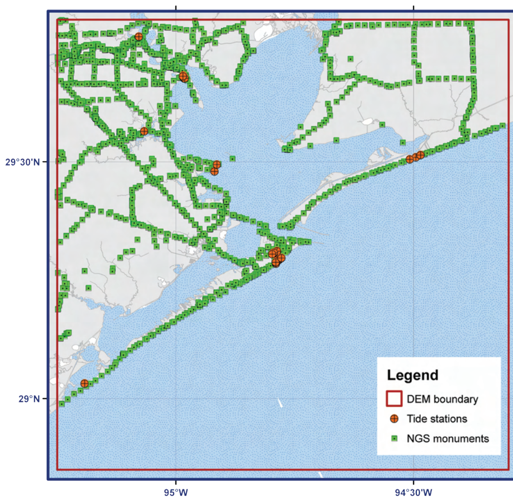
Figure 15. Location of NGS monuments and NOAA tide stations in the Galveston region. NGS monument elevations were used to evaluate the DEM.
