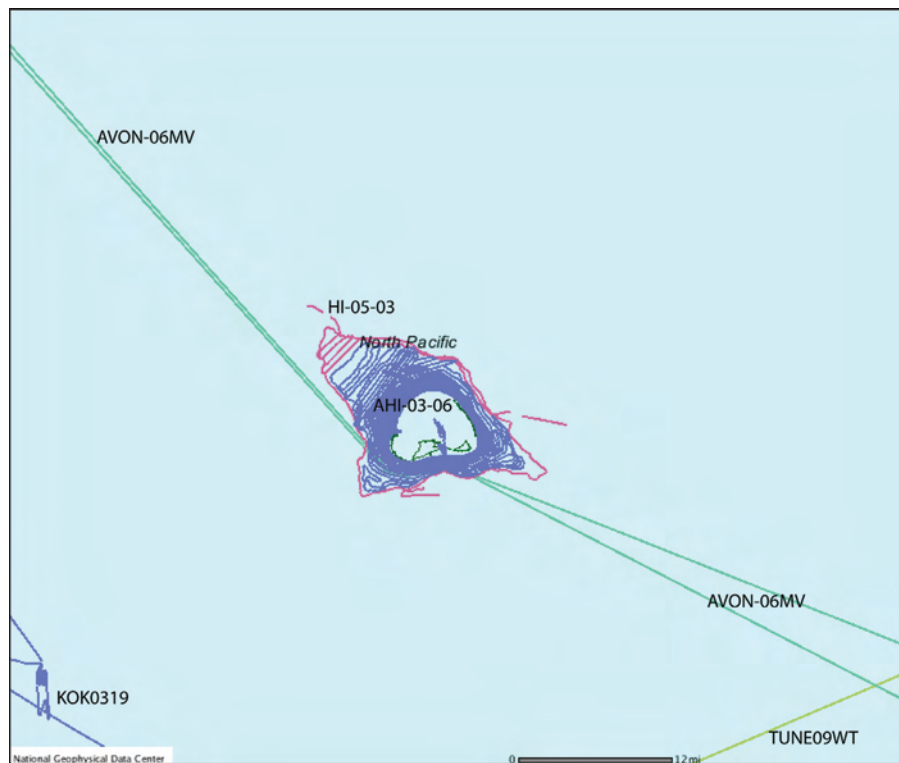
Figure 8. Ship tracks of multibeam swath sonar surveys used in compiling the Midway Atoll DEMs.
