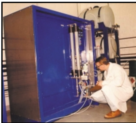
Bend Research's membrane-based solvent recovery system can dehydrate solvents, such as isopropyl alcohol, effectively to make recycling of aqueous- or alcohol-based solvents practical and cost effective.
