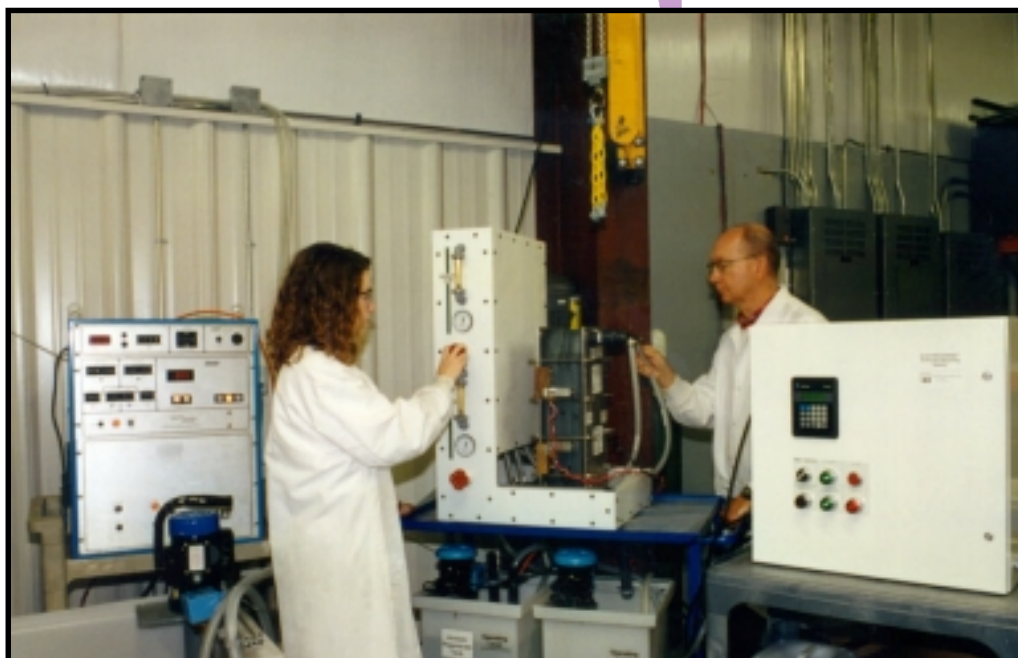
Faraday's E-Change™ In-Process Recycling System is capable of recycling approximately 90 percent of the contaminated electroplating rinse water back into the plating process, nearly eliminating metal sludges and significantly reducing water use.
