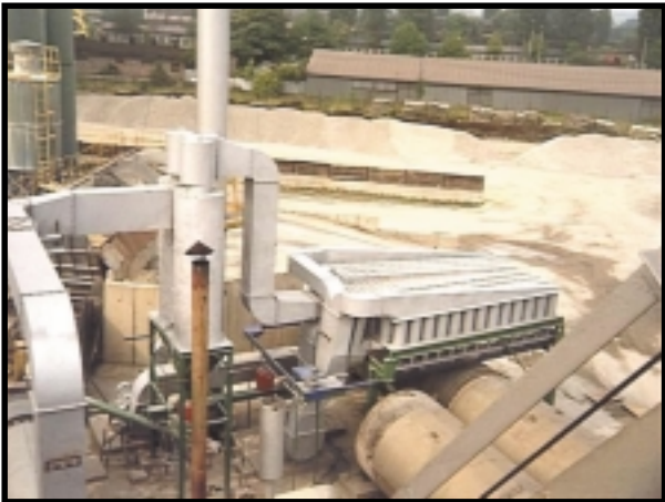
More than 50 Core Separators, such as the one at the asphalt plant above, have been installed in the United States and other countries to remove dust particles from gas streams.
