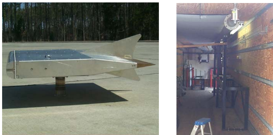
Figure 2-3. Plume Sampling System Probe (left) and Virtual Impactor Connected to the Sampling Tunnel (right)
