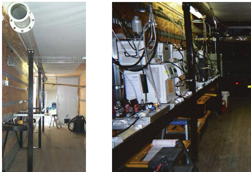
Figure 2-4. Photographs of the DEAL during Fabrication Showing Sampling Tunnel and Plume Bench (left), and with Instruments Installed (right)
