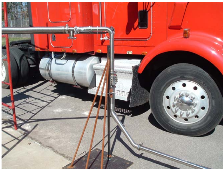
Figure 4-2. Line loss sample location at probe inlet.
