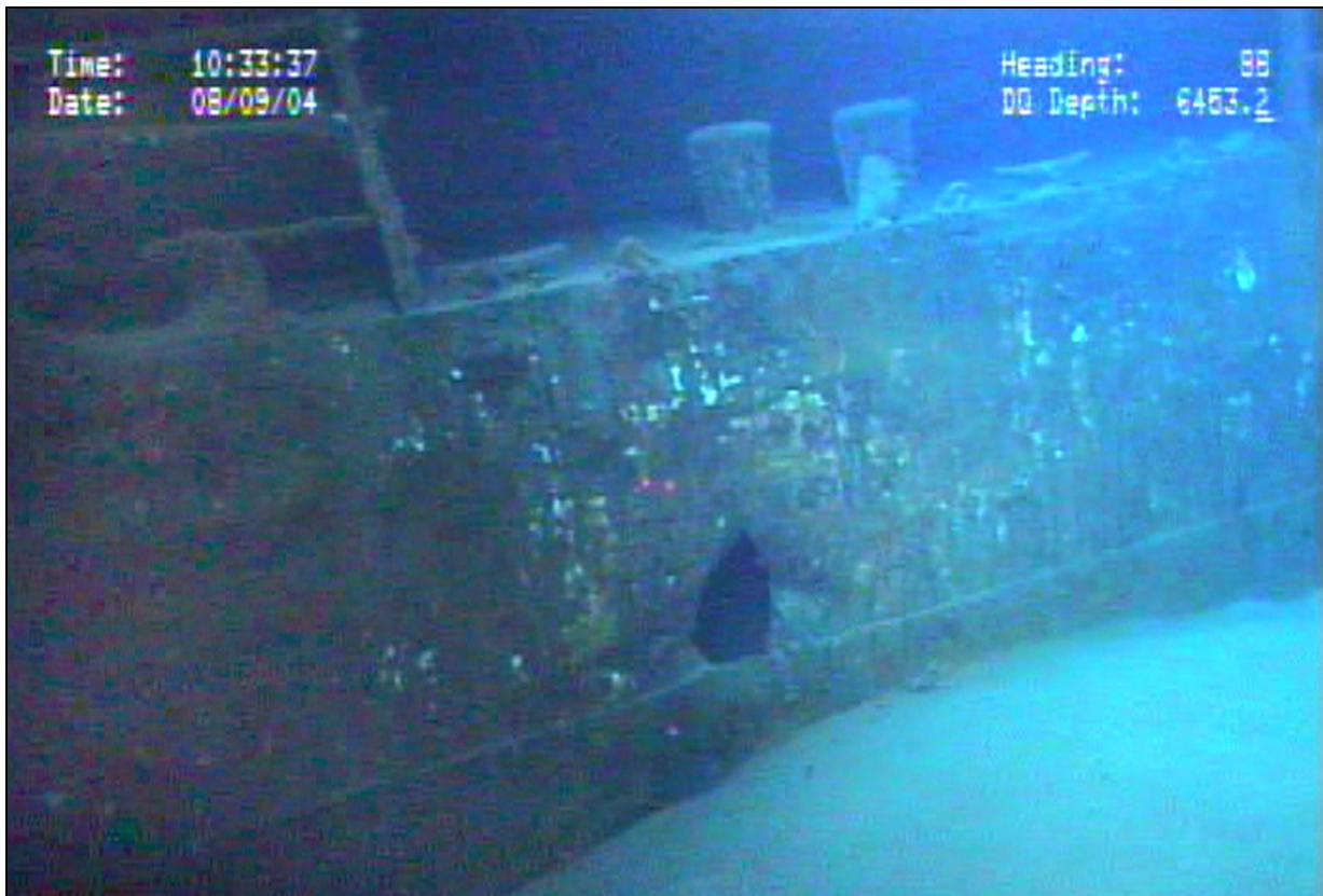
Figure 9.7. 105-mm shell damage on *Alcoa Puritan*'s starboard side. The breach is approximately 47 centimeters across.
