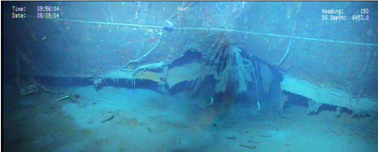
Figure 9.8. Mosaic of the vessel's port side torpedo damage just below the superstructure's aft section.
