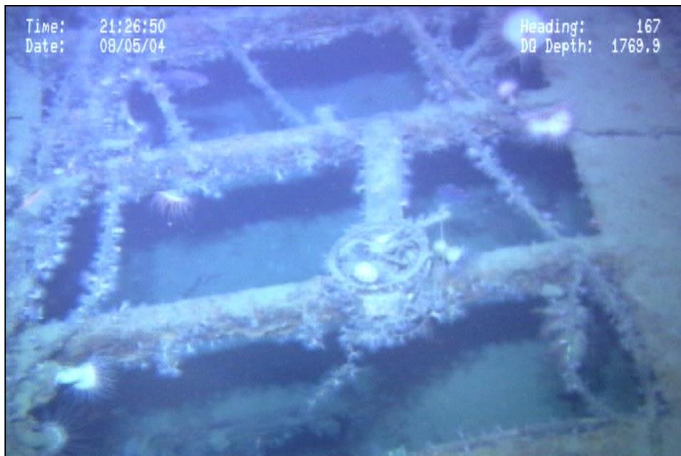
Figure 6.7. Top of *Gulfpenn*'s superstructure showing the bridge telegraph lying across the exposed deck frame supports.
