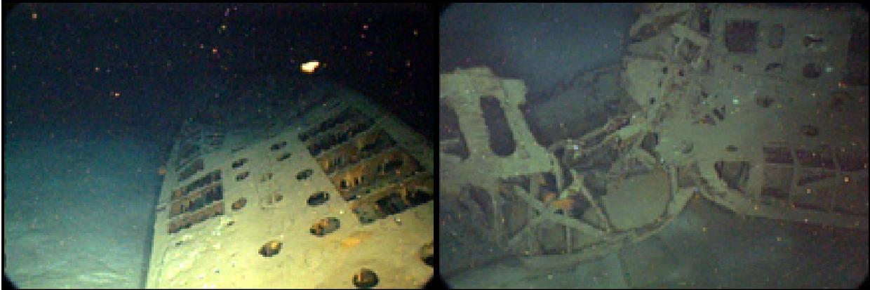
Figure 7.11. *U-166* images showing indentation (left) and damaged area near the forward torpedo-loading hatch (right).
