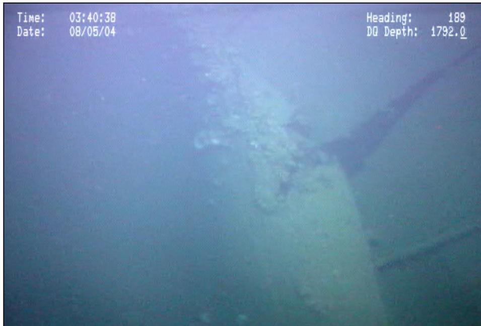
Figure 6.8. Breach in the hull along the vessel's starboard side.
