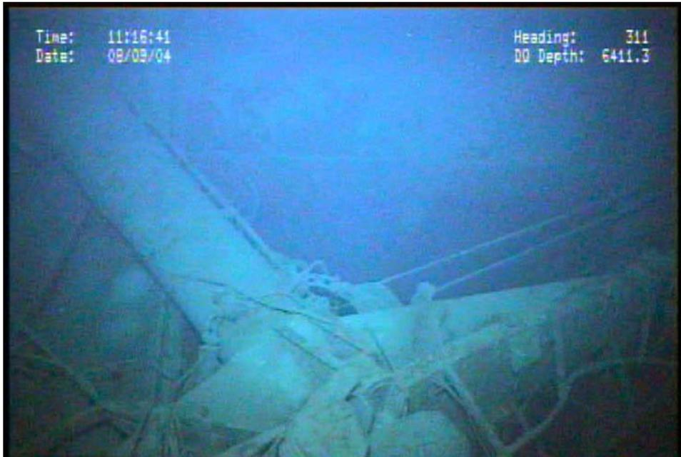
Figure 9.11. The top of the foremast lying over the No. 1 hold (looking aft).
