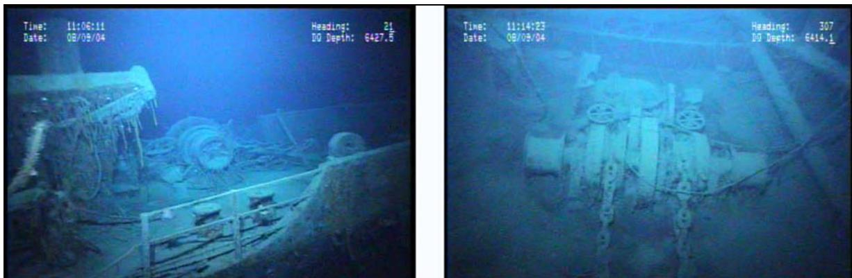
Figure 9.9. Two views of the ship's windlass: the view from starboard (left image), and the view from the bow looking aft (right image).
