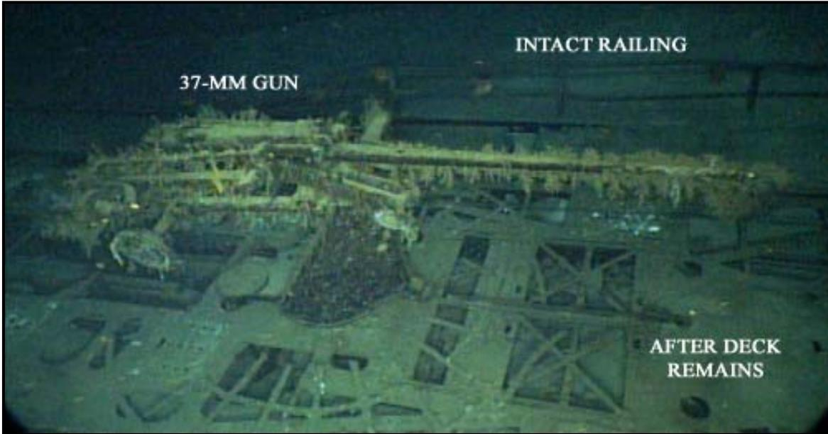
Figure 7.15. *U-166*'s aft deck of showing the 37-mm gun and intact deck railing.
