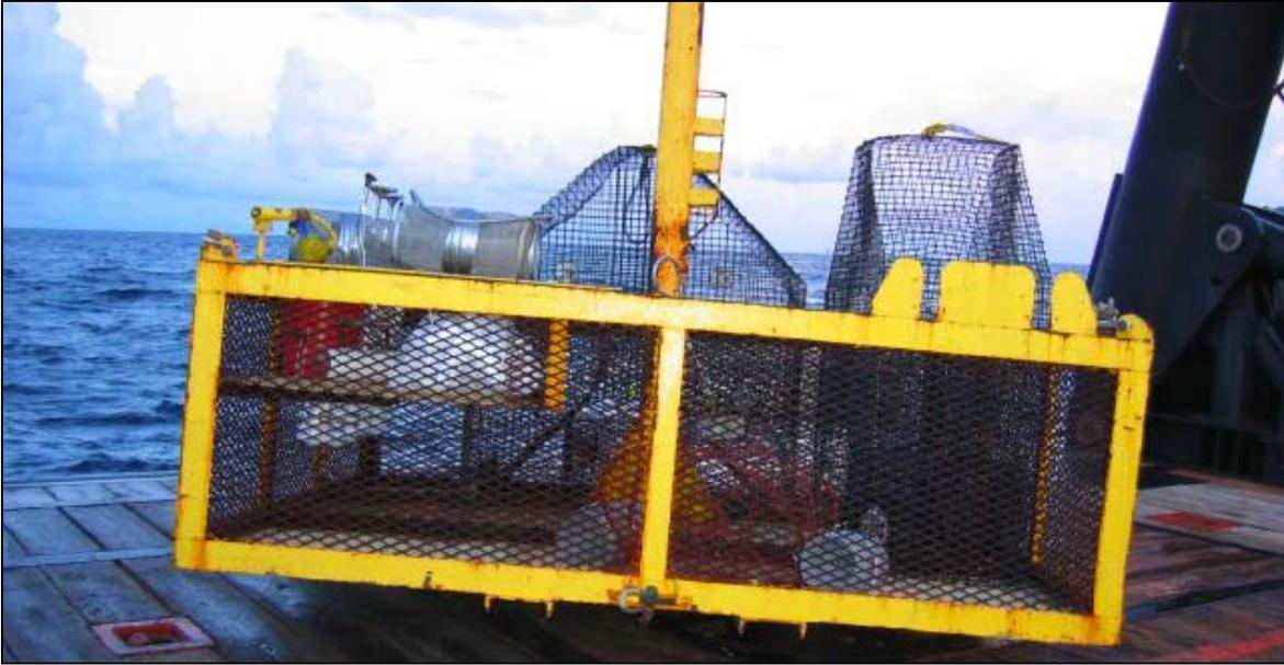
Figure 3.7. The vertebrate and invertebrate traps in the basket about to be lowered off the stern of HOS *Dominator*.
