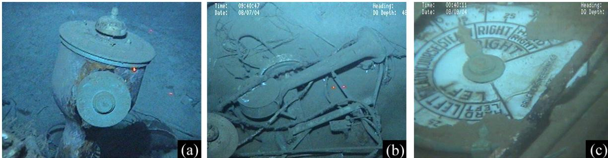
Figure 8.17. (a) Bridge signal bell, (b) Engine Order Telegraph lying across the Base of the Rudder Controls, and (c) Close-up of the Rudder Controls' Face.
