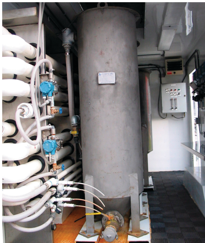
Pilot-scale Blue CAT™ equipment, including pre-reactor assembly on the left and reactive filter in the middle
