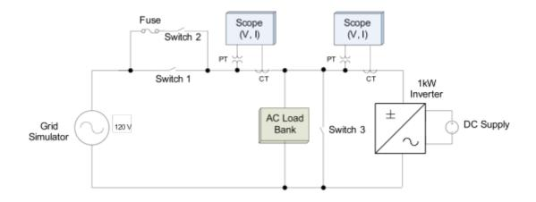
Figure 15. Test circuit single-line diagram
