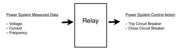
Figure 3. Input and output control of a protective relay
