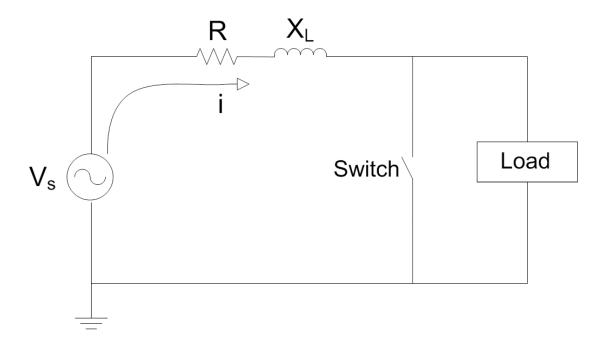
Figure 8. Circuit model for asymmetrical fault current
