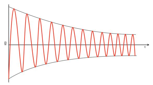
Figure 9. AC symmetrical short-circuit current
