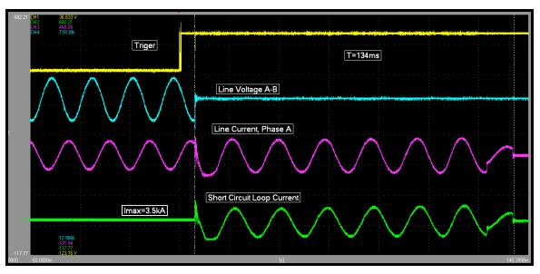
Figure 28. Manufacturer testing inverter for voltage ride-through
