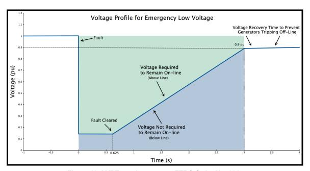
Figure 19. LVRT requirement per FERC Order No. 661
