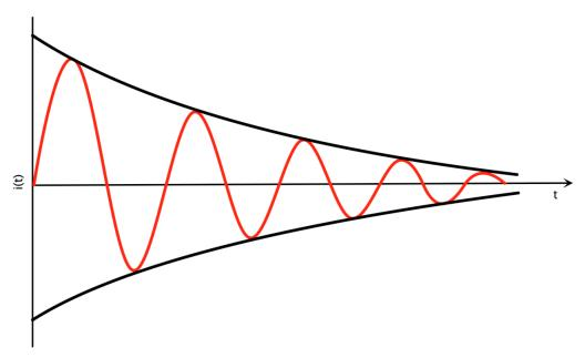
Figure 13. Induction machine response to 3-phase fault
