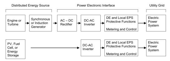
Figure 14. DER system and PE interface block diagram (Kroposki et al. 2006)
