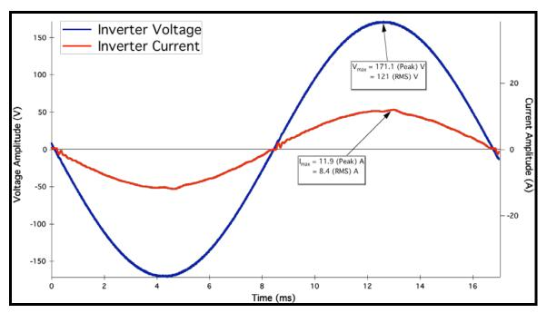
Figure 16. Pre-fault waveform of 1 kW inverter
