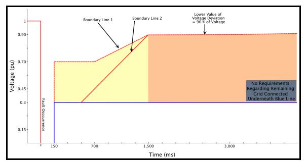
Figure 26. Germany's new LVRT grid code
