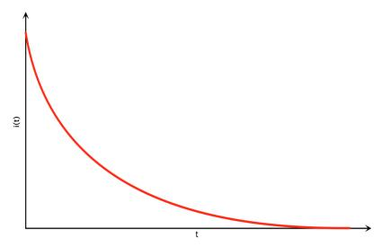
Figure 10. Decaying DC offset short-circuit current
