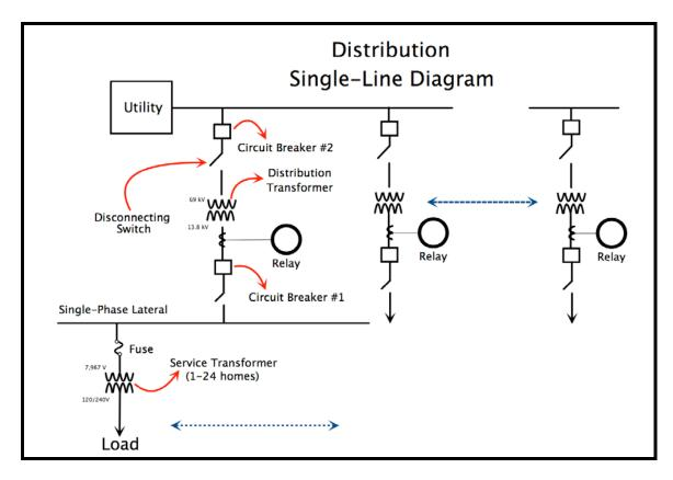
Figure 7. Typical single-line diagram
