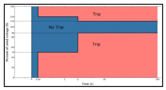
Figure 25. IEEE 1547 Interconnection system response to abnormal voltages from IEEE 1547 (Table 1)
