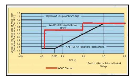
Figure 21. 2005 WECC LVRT standard (Zavadil et al. 2005)
