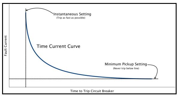
Figure 6. Example of a time current curve
