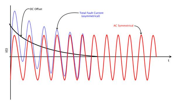
Figure 11. Total (DC and AC components) short-circuit asymmetrical current
