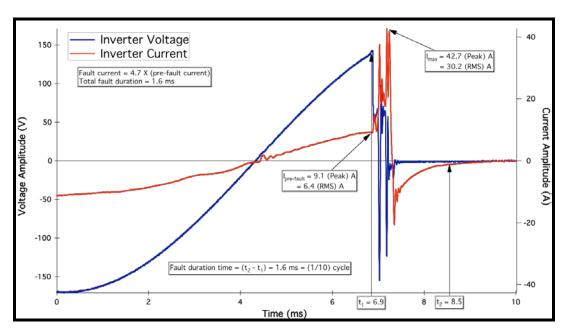
Figure 17. Fault current test result of 1 kW inverter
