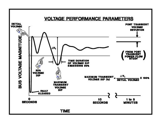
Figure 20. WECC system performance criteria from Table W (WECC System Performance Criteria, TPL – WECC – 1 – CR, 2008)
