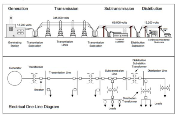
Figure 2. Typical electric power system single-line diagram
