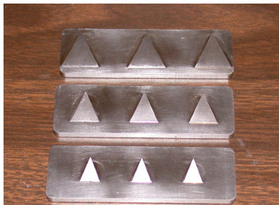
Figure 5.—Picture of three microramp inserts.
