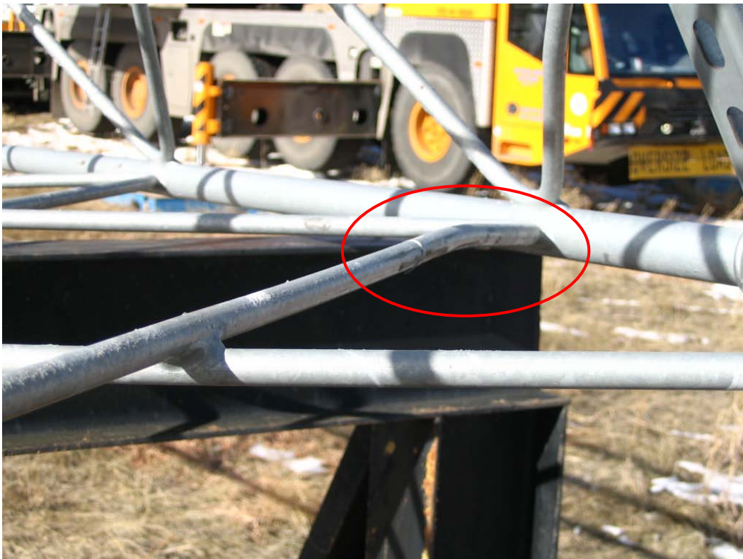
Figure C-16. Bent tower diagonal
