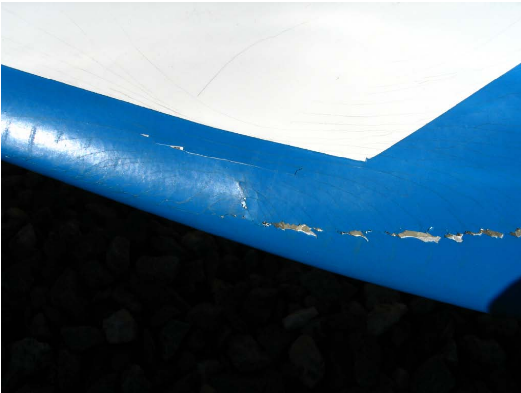
Figure C-12. Crack in leading edge of blade #2
