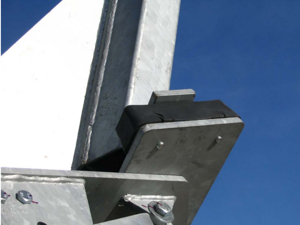
Figure C-13. Cracked tail stop bumper
