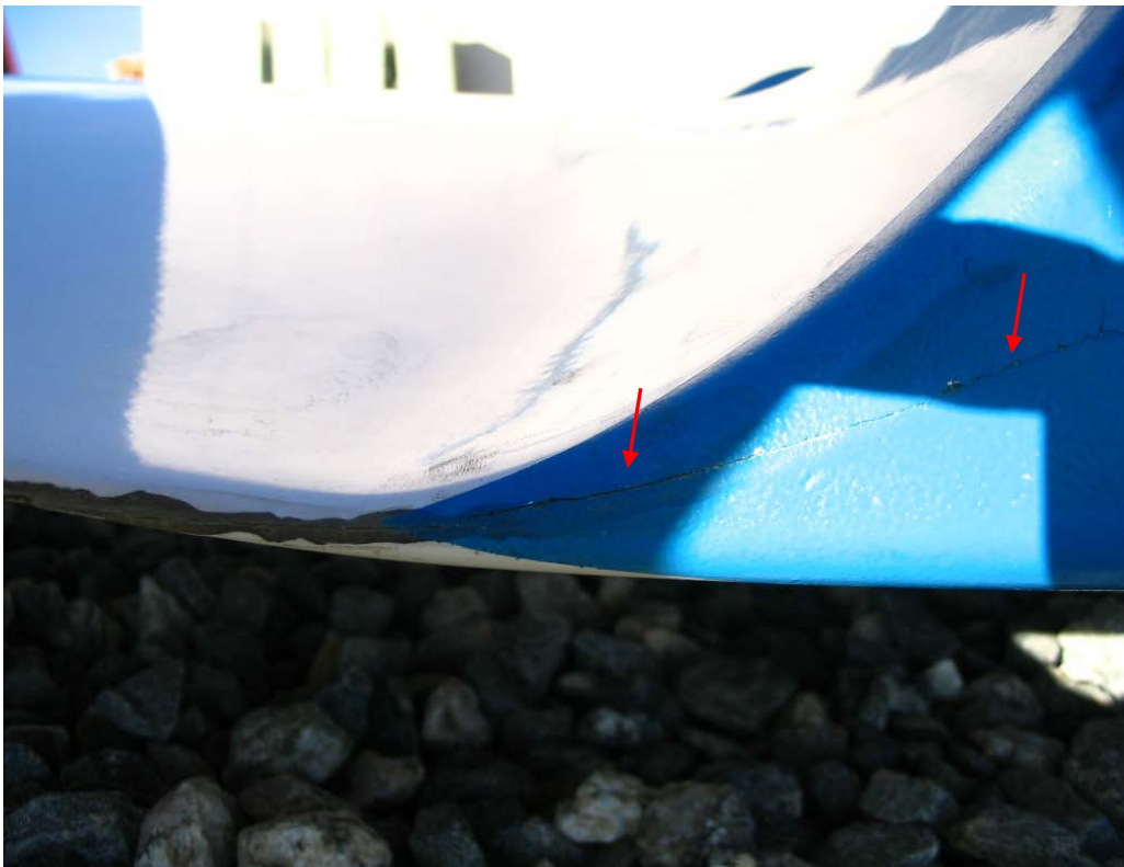
Figure C-10. Crack in trailing edge of one of the blades
