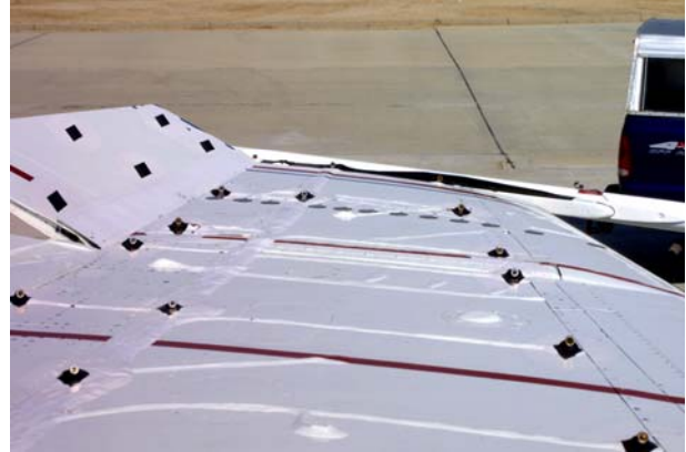
Figure 17: Black diamond targets on AAW F/A-18.
