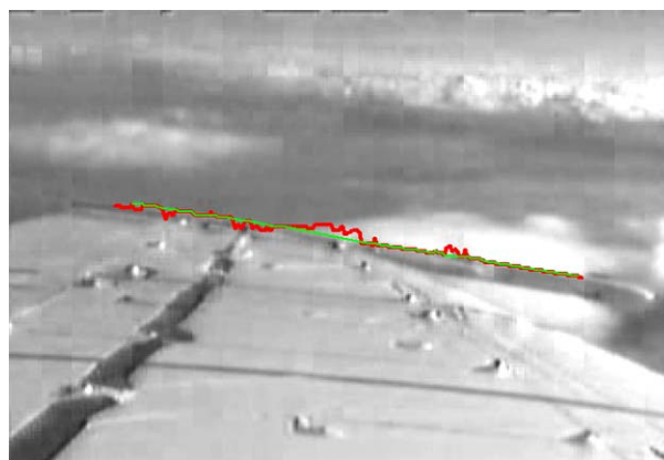
Figure 8: Detection of upper edge of launcher rail with image processing
