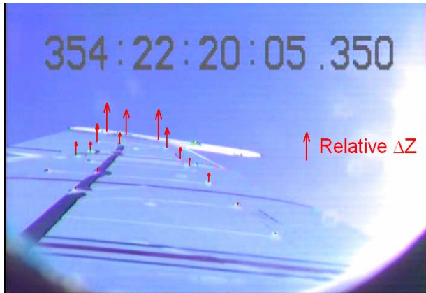
Figure 9: Relative Z-deflection overlaid on video image of wing.
