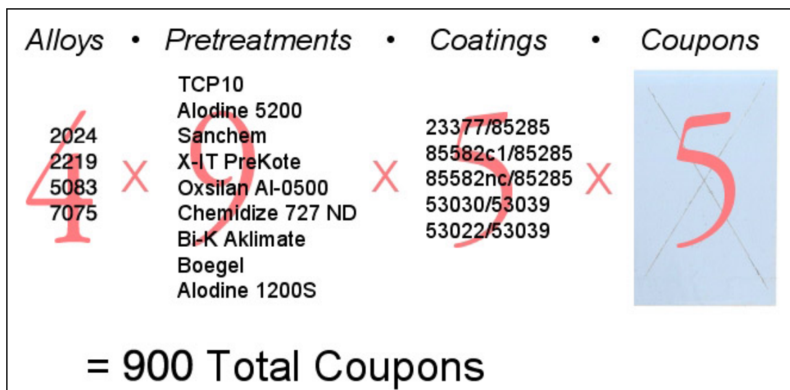
Figure 1. ASTM B 117 test panel matrix breakdown.
