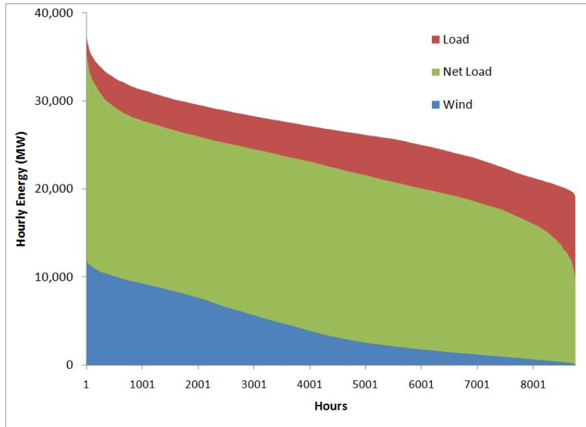
**Figure 3 – Adding wind accentuates the “peaky” nature of the load duration curve.**
