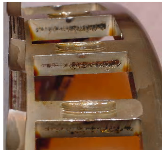
Figure 12.—Test 2 cage damage at test completion.
