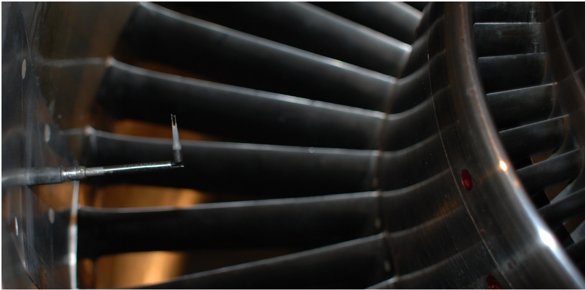
Figure 5.—Photograph of a hot-film probe installed in the NASA Fan model.
