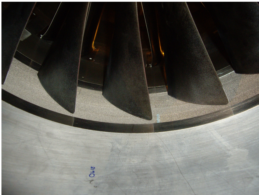
Figure 2.—The FeCrAlY metal foam OTR treatment with no perforate cover sheet as installed in the ADP model.
