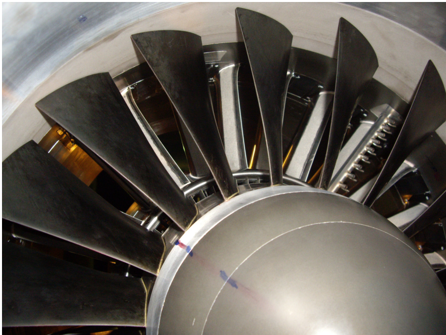
Figure 4.—The soft stator vanes behind the rotor in the ADP model.
