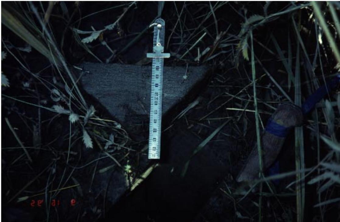
Figure 11. Wedge-shaped sediment block used to measure vertical accretion. Note subhorizontal laminations.
