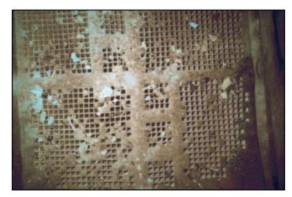
Plugging that may occur during normal operations of an SCR facility
