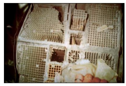
Damage caused by erosion in the catalyst bed
