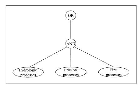
Figure 6—Network for **watershed processes**. The truth of the proposition that watershed processes are within a suitable range of conditions depends on the degree to which its three premises, represented by the networks **hydrologic processes**, **erosion processes**, and **fire processes**, are true.
