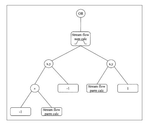
Figure 8—Network for **stream flow**. The rounded box represents a fuzzy curve that is dynamically defined. The fuzzy curve object compares the value of **stream flow sum calc** (fig. 9) to the x coordinates in its xy nodes to interpolate the truth value for **stream flow**. The calculated data link, stream flow calc, computes the sum of the weights for terms in fig. 9 to dynamically define the x coordinates of the xy nodes.
