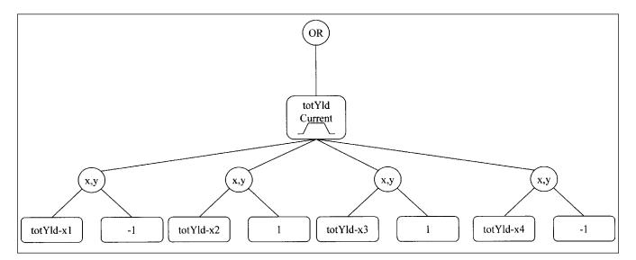
Figure 10—Network for **total water yield** from the watershed. The rounded box represents a fuzzy curve that is dynamically defined. The fuzzy curve object compares the value of **totYldCurrent** to the x coordinates in its xy nodes to interpolate the truth value for **total yield**. The x terms in each xy node are calculated data links (fig. 11).
