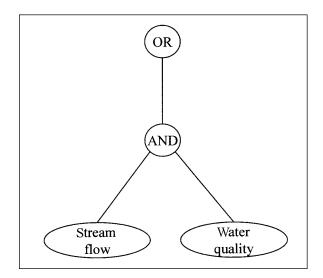
Figure 7—Network for **hydrologic processes**. The truth of the proposition that hydrologic processes are within a suitable range of conditions depends on the degree to which its two premises, represented by the networks **stream flow**, and **water quality**, are true.
