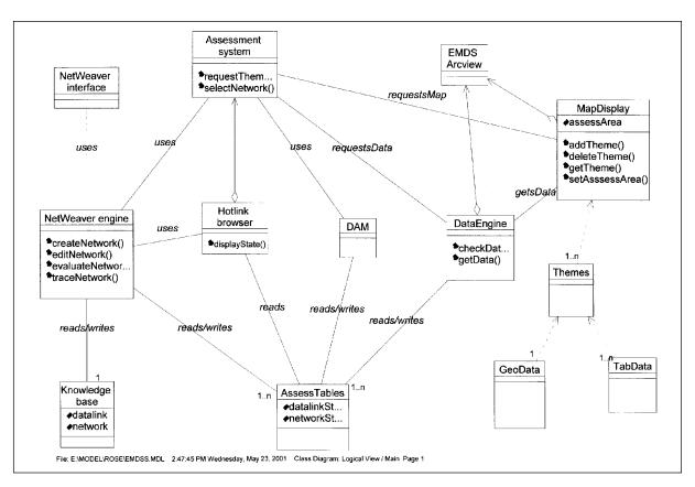
Figure 2—Object diagram of the ecosystem management decision-support system.
