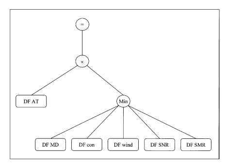
Figure 13—Network for evaluating yield suitability of Douglas-fir in Great Britain. **AT, MD, con, wind, SNR** and **SMR** indicate computational networks that compute site indices for accumulative air temperature, moisture deficit, continentality, wind, soil nutrient regime, and soil moisture regime, respectively, for Douglas-fir.
