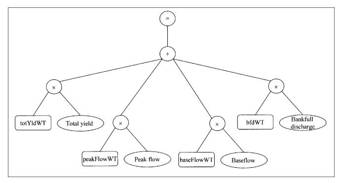
Figure 9—Calculated data link for stream flow sum calculation. The calculated data link computes a sum of products. The weights for each term in the sum are read as data.
