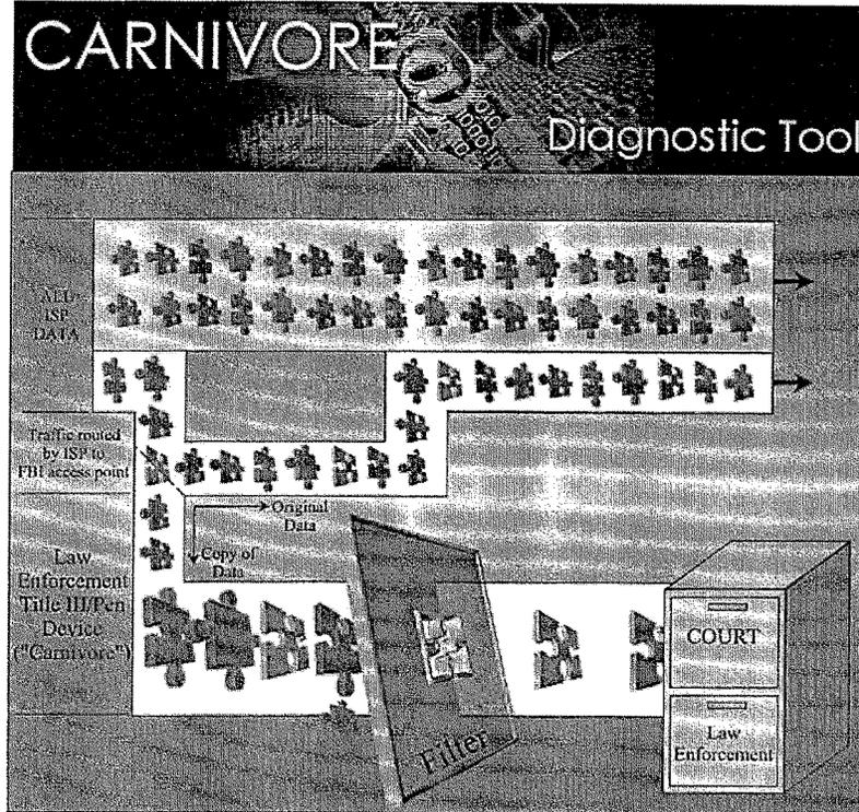
The top of the diagram shows all traffic through an Internet Service Provider (ISP). The FBI and ISP work together to identify an access point that contains all traffic from the suspect named in the court order, with as little other traffic as possible. In some cases, the ISP is able to provide the FBI with an access point that contains only the suspect's traffic.
