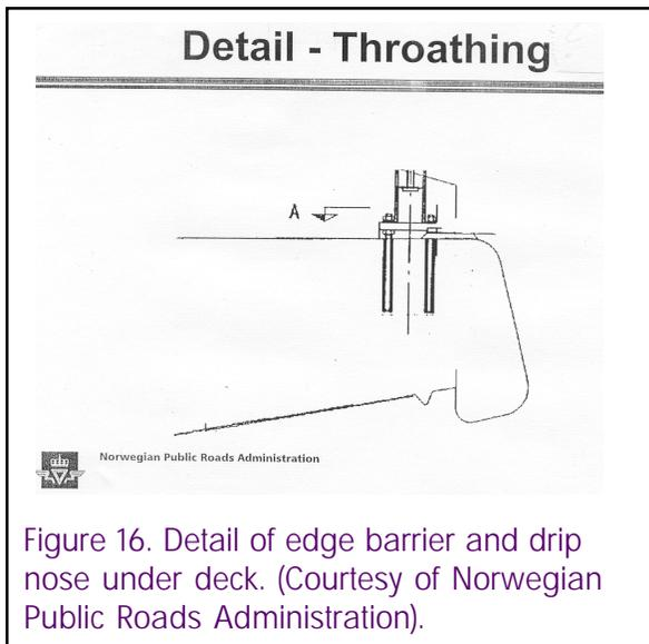
Figure 16. Detail of edge barrier and drip nose under deck. (Courtesy of Norwegian Public Roads Administration).
