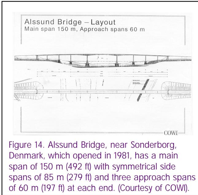
Figure 14. Alssund Bridge, near Sonderborg, Denmark, which opened in 1981, has a main span of 150 m (492 ft) with symmetrical side spans of 85 m (279 ft) and three approach spans of 60 m (197 ft) at each end. (Courtesy of COWI).
