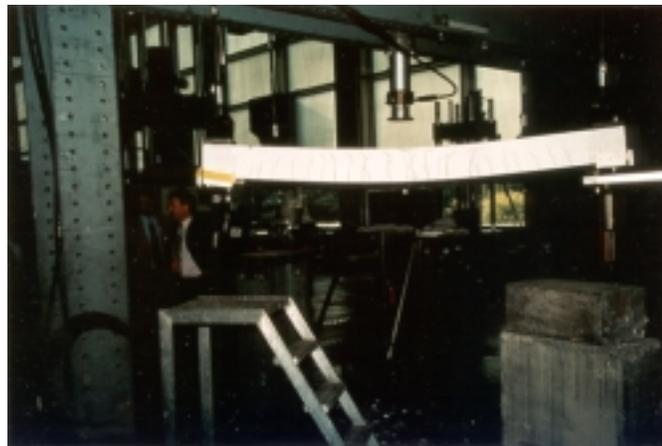
Figure 43. Fiber-reinforced concrete slab test at Swiss Federal Institute of Technology (ETH).
