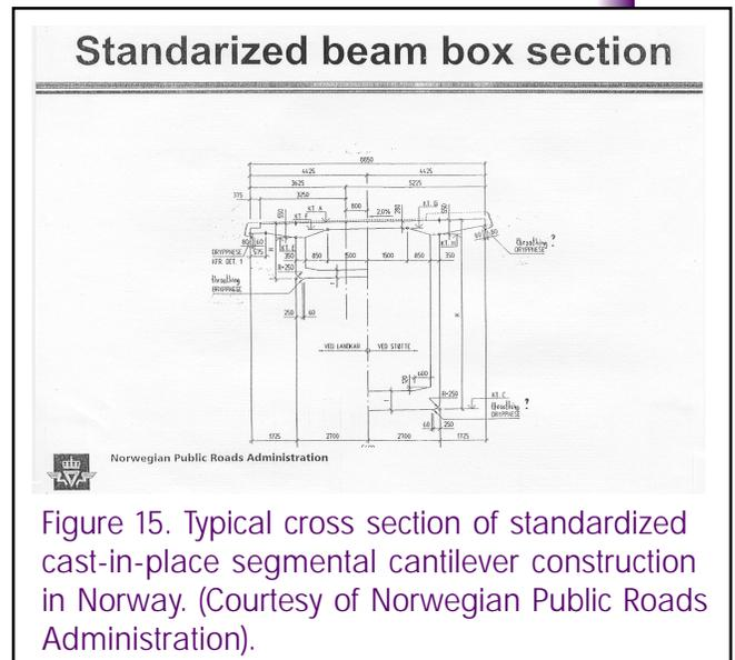
Figure 15. Typical cross section of standardized cast-in-place segmental cantilever construction in Norway. (Courtesy of Norwegian Public Roads Administration).
