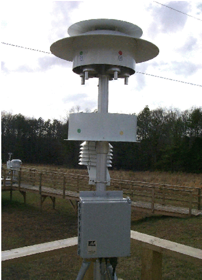
Figure I-2b. Picture of MetOne Sampler Deployed in the Field at RTP. Left – Inlet, Filter Holders, and Meteorological Sensor. Right-Pump box.
