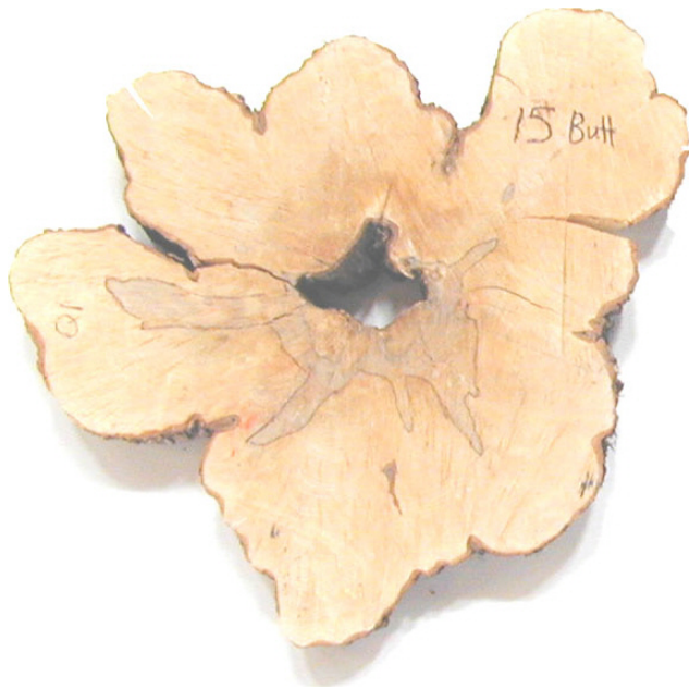
Figure 4.—Stump disk of sugar maple, showing irregularity in disk shape, and extreme irregularity in heartwood shape.
