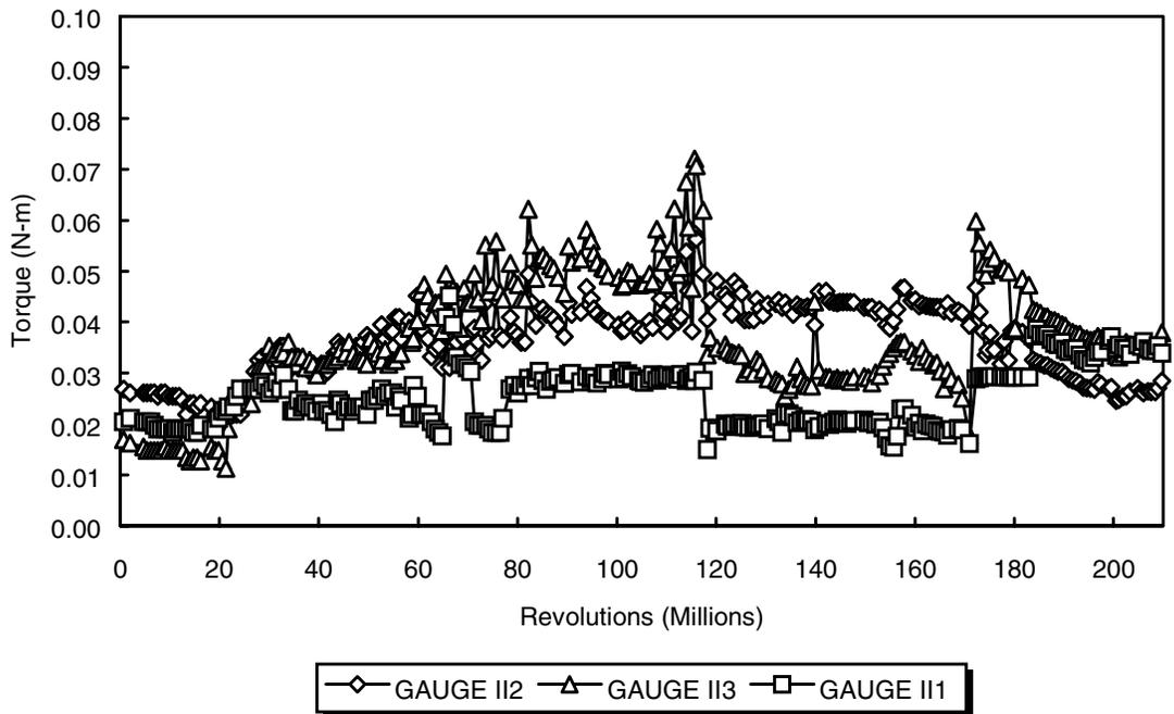
Figure 3 – Torque vs. revolutions for upper pair bearings (I11), middle bearings (I12), and lower bearings (I13)
