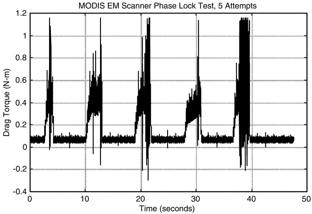
Figure 16 – MODIS EM Scanner Phase Lock Test 1
