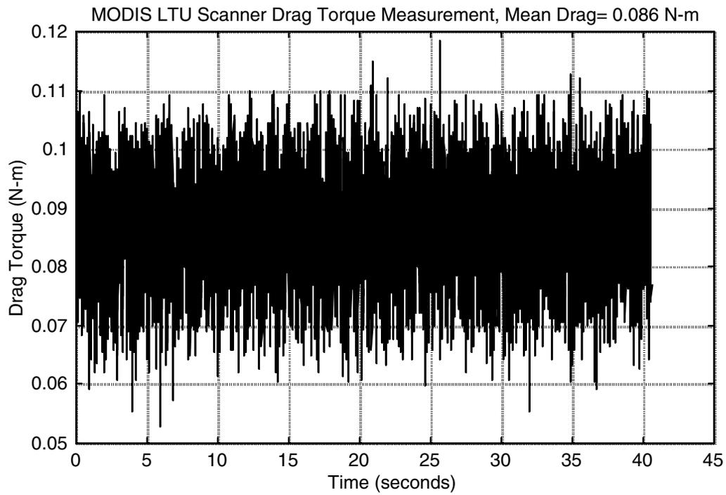
Figure 18 – MODIS LTU Scanner Steady State Drag Torque
