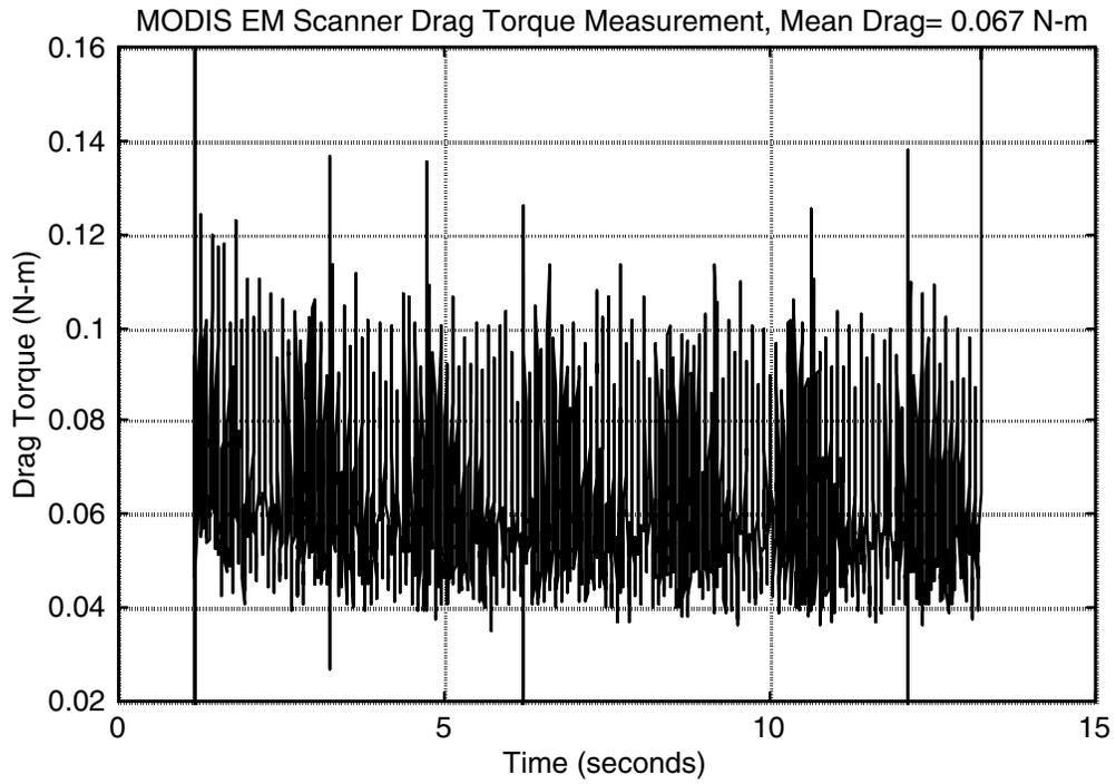
Figure 14 – MODIS EM Scanner Steady State Drag Torque
