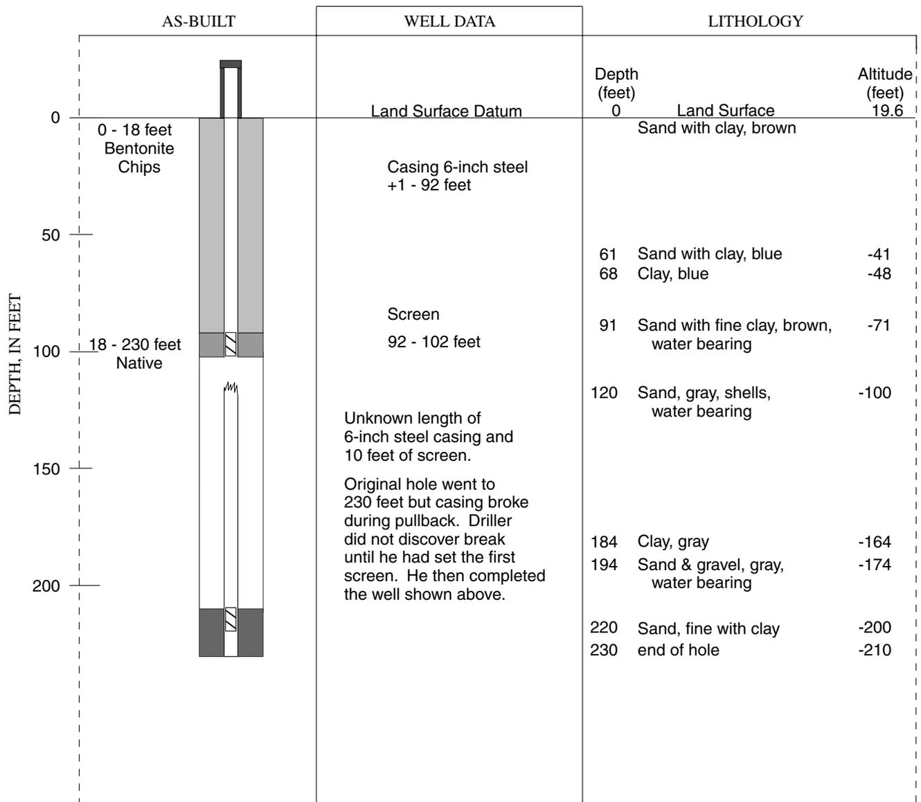
**Figure 3.** Construction, completion and generalized lithologic data for newly constructed tribal wells 14N/11W-02C01, 14N/11W-02C02, and 14N/11W-03F01.
