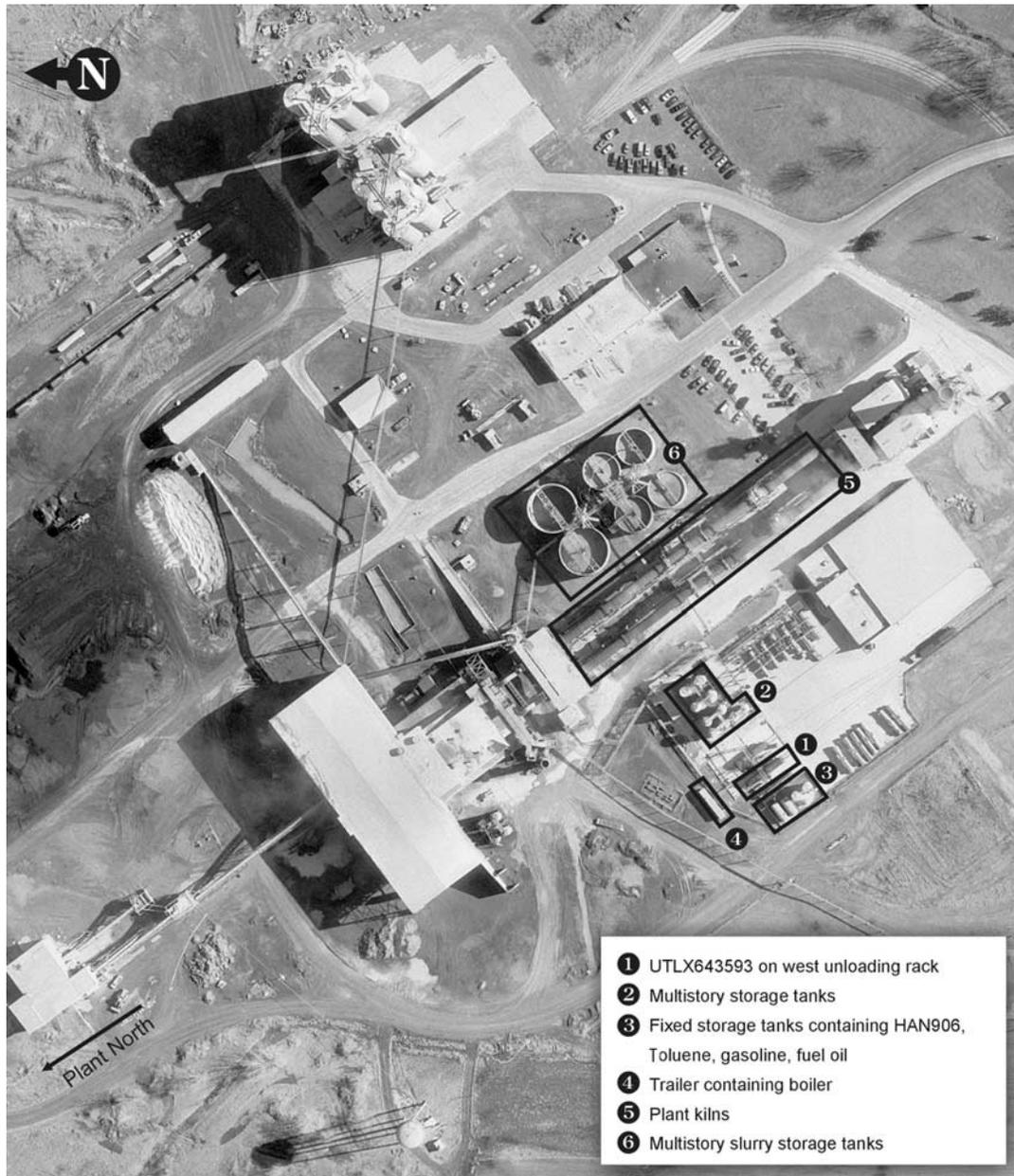
**Figure 2.** Aerial view of Essroc plant (preaccident); areas of interest cited in report are labeled. (Photo provided by Essroc)
